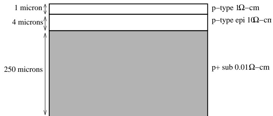
Figure 3.1. Doping profile of the heavily doped substrate.
