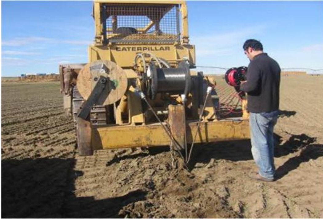
44 Figure 1 Photograph from September 2007 showing the “lift-plow” in operation.
