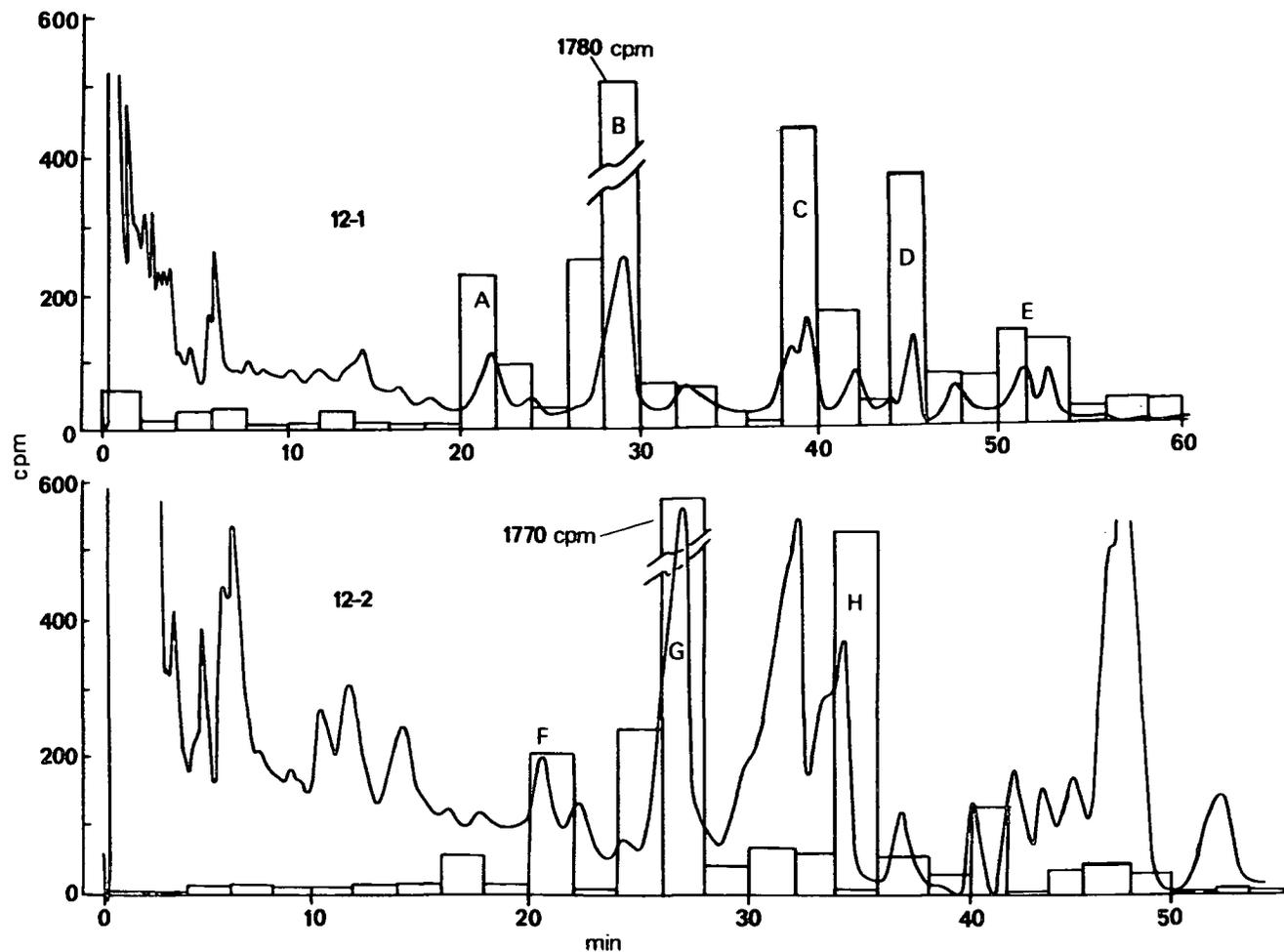
Figure 12. Gas chromatograms of rat urine (12-1) and fecal (12-2) methylated ether extracts on a 8' x 1/8" 10% Dega-PS column. Radioactivity in the effluent, collected in silicon-celite traps (Appendix X), is shown corresponding to the elution time. Peaks in the chromatograms containing significant radioactivity were assigned letters A through H.
