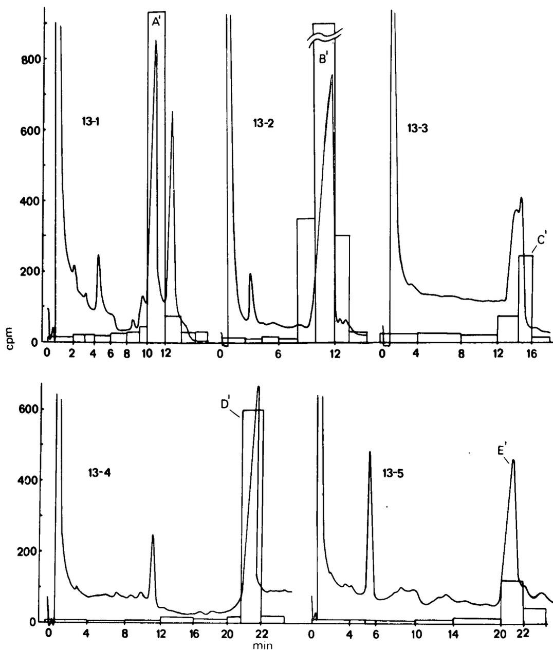
Figure 13. Gas chromatograms of radioactive peaks A through E in Figure 12 on a 8' x 1/8" OV-25 column. Radioactivity in the effluent, collected in silicon-celite traps (Appendix X), is shown corresponding to the elution time. Peaks in the chromatograms containing significant radioactivity were assigned letters A' through E'.
