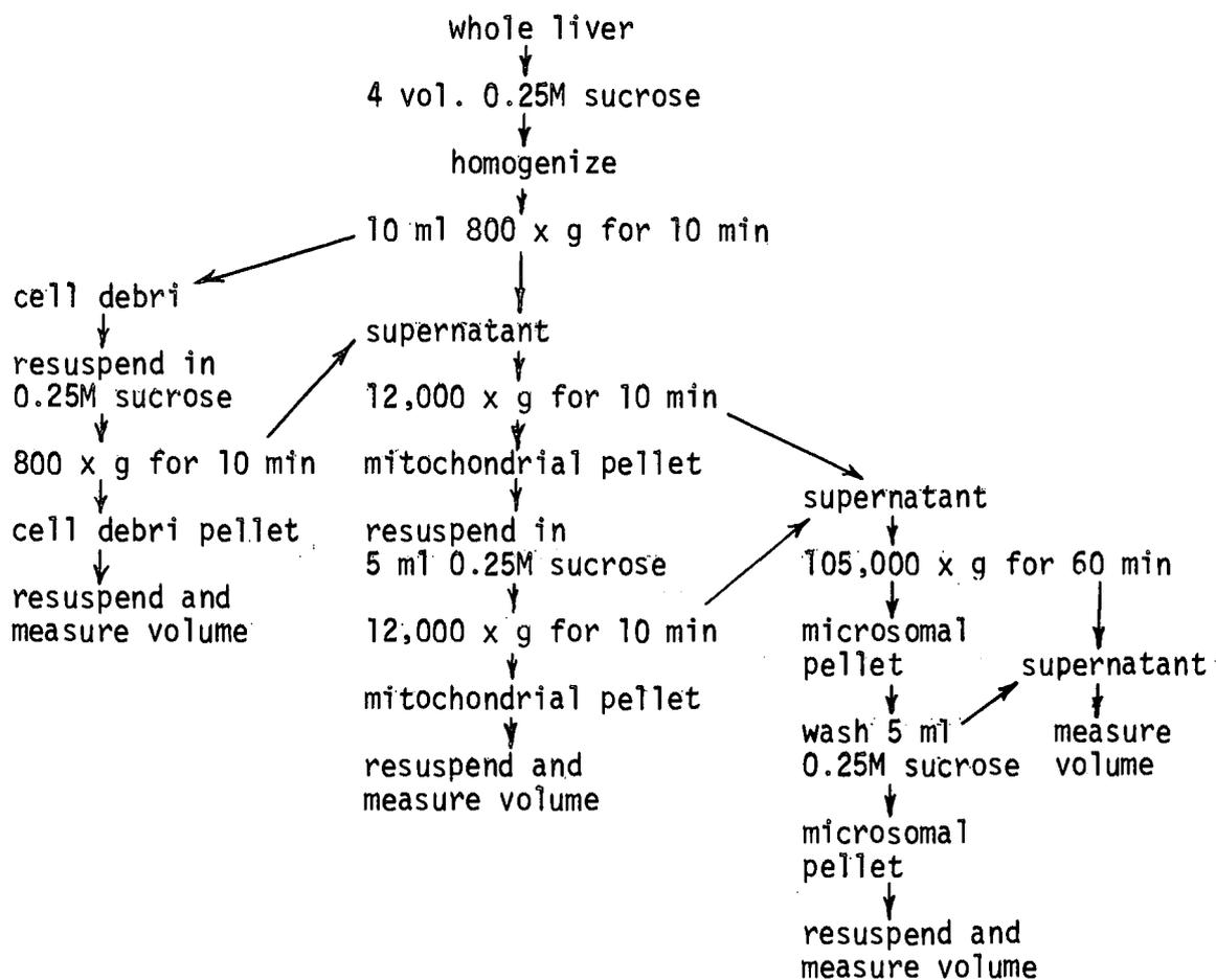
Figure 3. Flow diagram of liver subcellular fractionation procedure.
