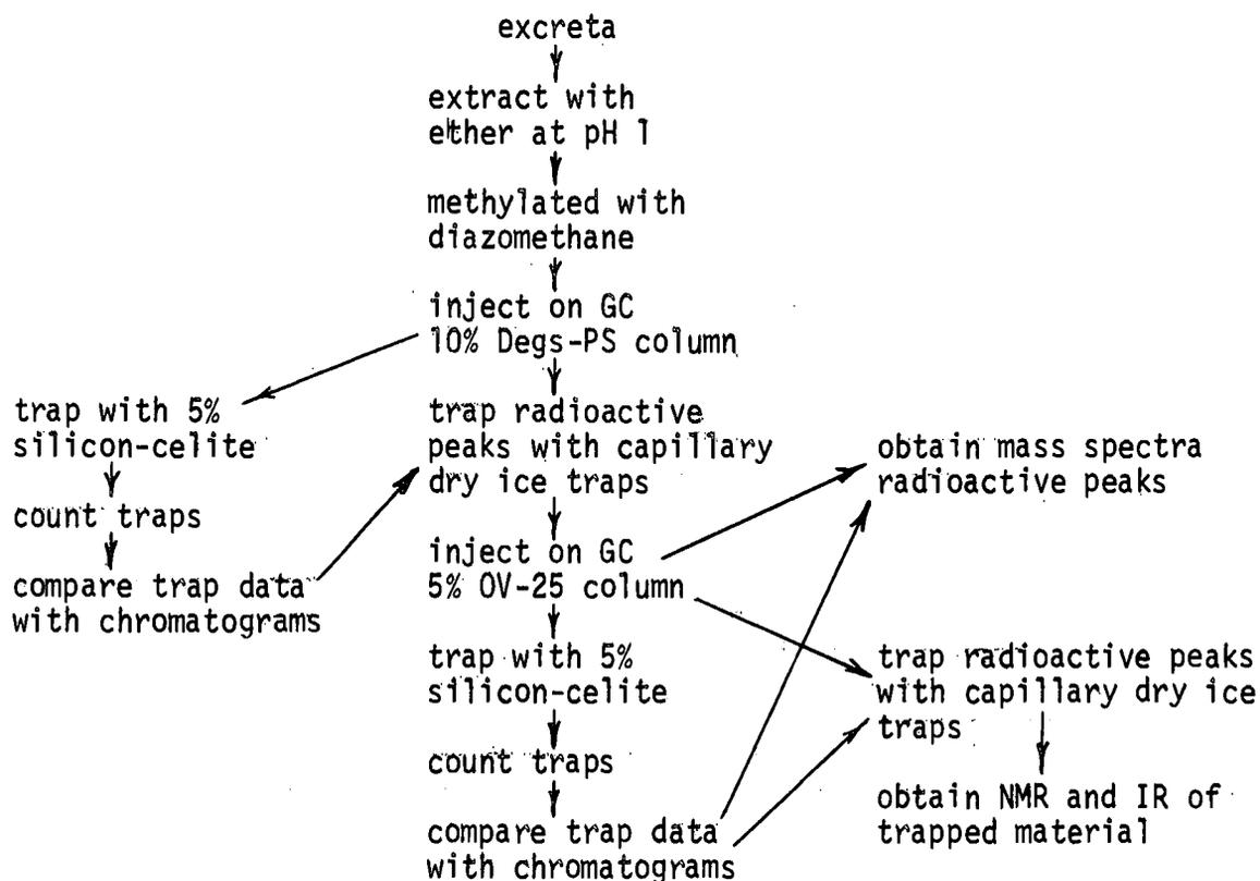
Figure 5. Flow diagram of metabolite isolation procedure.
