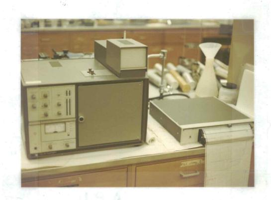
Figure 1. Hewlett-Packard Model 5710A gas chromatograph.
