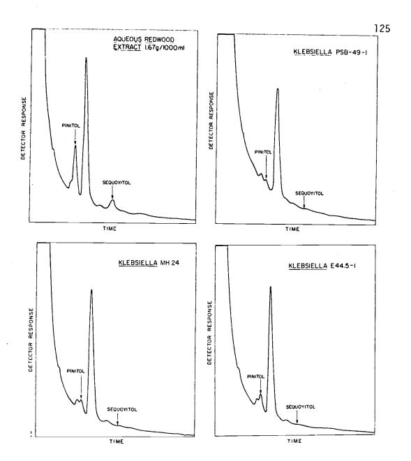
Figure 3. Gas chromatographic analysis of cyclitol utilization by <u>Klebsiella</u> in a 1.67 g sawdust/ 1000 ml water extract of redwood. Column temperature was 160°C. Origin of isolates tested: PSB49-1, mastitis; MH24, vegetable; E44.5-1, redwood.
