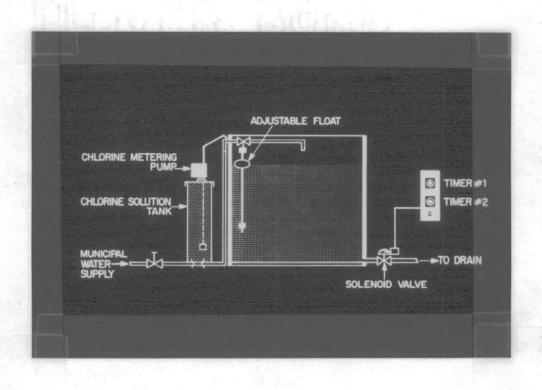
Figure 2. Diagram showing design modifications included in the 1,000 gal (3,788 1) experimental tank.
