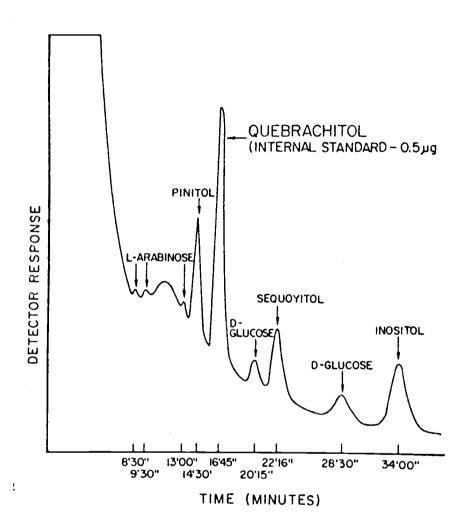
Figure 4. Analysis of the sterile minimal salts medium containing two carbohydrates and three cyclitols as carbon sources. Column temperature was 145°C for 8 minutes, then with heating at 4°C/min., to 160°C. The change in baseline after 9'30" is a reflection of the increase in column temperature.
