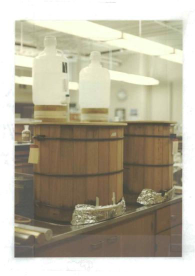
Figure 1. 90 liter redwood reservoirs used in these experiments.
