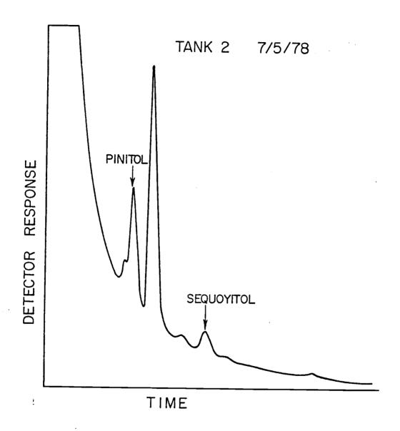
Figure 5. Tank 2 water collected on 7/5/78 (stagnant tank). Column temperature was 160°C.
