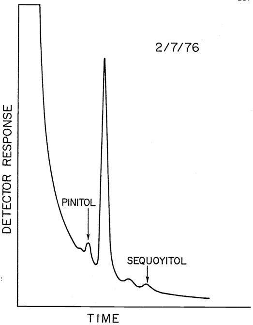
Figure 3. Analysis of sample taken from the experimental reservoir on 2/7/76. Column temperature was 160°C.
