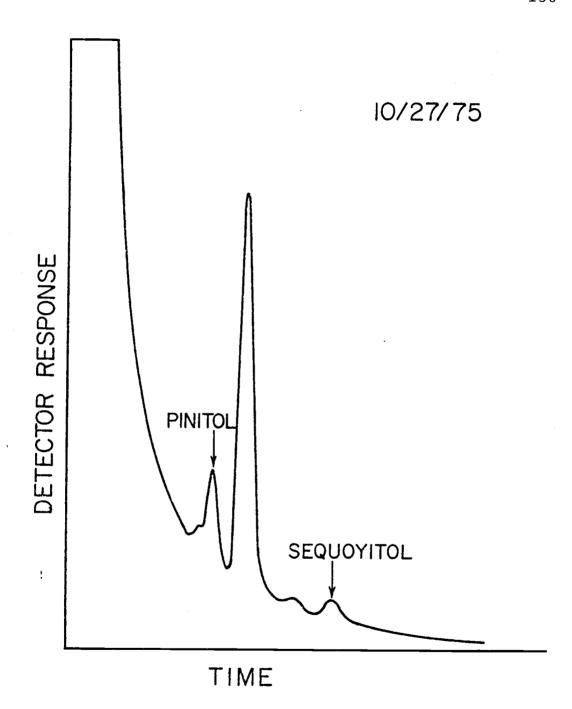
Figure 2. Gas chromatographic analysis of a sample taken from the experimental redwood water reservoir on 10/27/75. Column temperature was 160°C.
