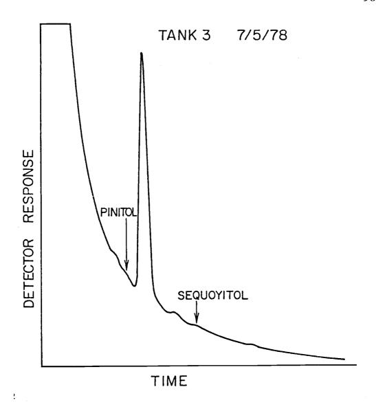
Figure 7. Tank 3 water collected on 7/5/78 (8 day retention). Column temperature was 160°C.
