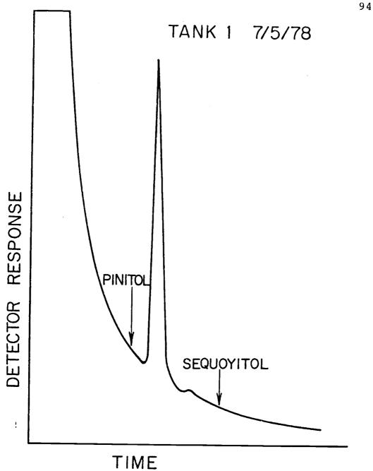
Gas chromatographic analysis of tank 1 water collected on 7/5/78 (3 day retention schedule). Figure 3. The large peak is that of quebrachitol, the internal standard. Column temperature was 160°C.
