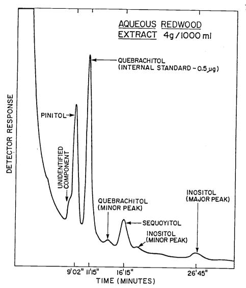
Figure 2. Gas chromatographic profile of a 4 g sawdust/ 1000 ml water extract of redwood sawdust. Column temperature was 160°C.
