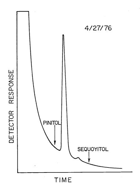
Figure 4. Analysis of sample taken from the experimental reservoir on 4/27/76. Column temperature was  $160\,^{\circ}\text{C}$ .
