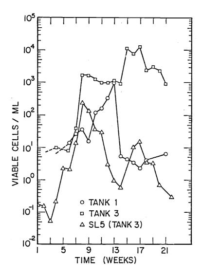
Figure 8. Klebsiella densities observed in water stored in redwood tanks 1 and 3. Included are densities for Klebsiella SL5, an antibiotic resistant culture.
