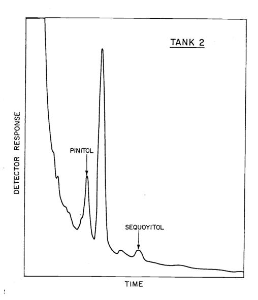
Figure 4. Analysis of tank 2 water collected on 3/14/78 (8 day retention). Column temperature was 160°C.
