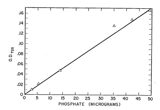
Figure 2. Plot of inorganic phosphate vs. absorbance at  $725~\mathrm{nm}$ .
