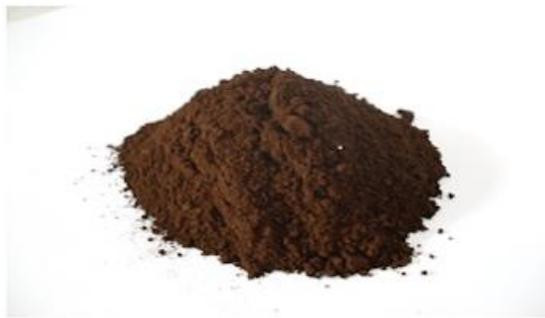
**Figure 1.1:** Dark brown lignin powder for bench-scale experiments between 1.35 and 1.50 [2]. It is not completely soluble in water because the hydroxyl group can form strong hydrogen bonding to prevent lignin dissolution. After further degradation, lignin becomes soluble in the mixture of water and organic solvents. Its solubility depends on many factors such as plant species, types of condensation reaction, and methods of lignin degradation or fractionation.
