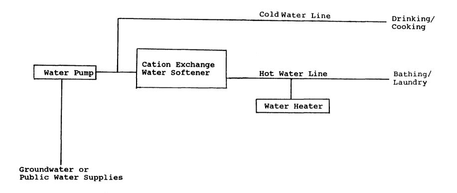
Figure 2. Separate Water Line System
