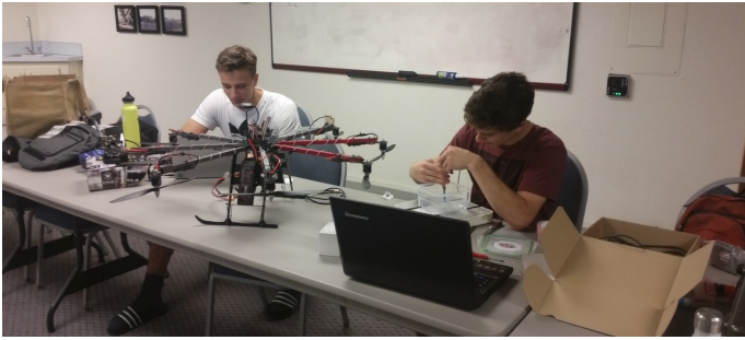
Fig. 15: Primary author, Brett (right), working alongside Jonah Siekmann (left) to attach the RFID reader antenna onto a octocopter drone– an effort that turned out to be only semi-successful due to a design flaw in the drone and RFID read range limitations.
