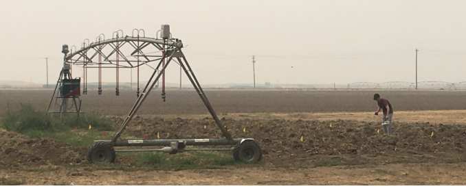
Fig. 11: Image from the field trial, taking place on a 10 meter radius center pivot irrigation arm.
