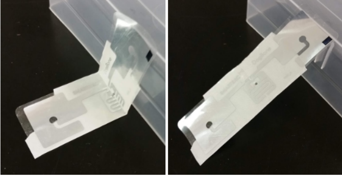
Fig. 2: The RFID tag was shown to exhibit different moisture values when flat and curved (21 and 31 respectively)
