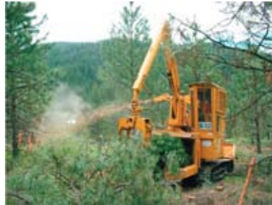
Figure 6. Whole-tree chipper in pine stand.
