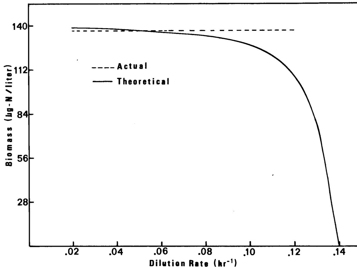
Figure 24. Theoretical and observed nitrogen biomass at steady state as a function of dilution rate.
