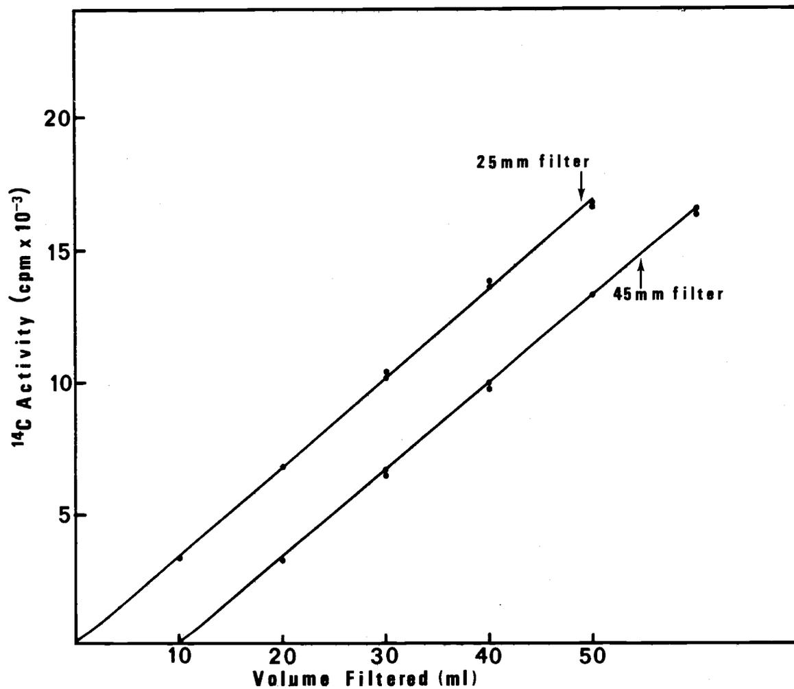
Figure 7. Relationship between  $^{14}\text{C}$  activity and volume of culture filtered indicating lack of appreciable self absorption. Axis was shifted to the right for the 45 mm filter experiment.
