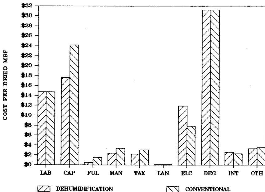
Figure 5. Cost factor breakdown
