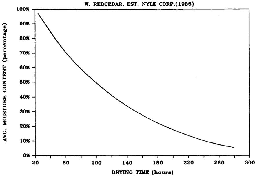
Figure 3. Dehumidification drying curve
