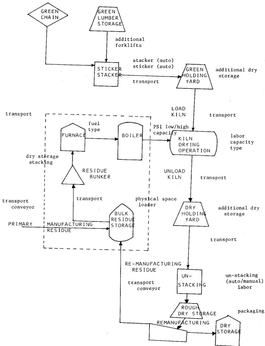
Figure 1. Proposed lumber drying operation
