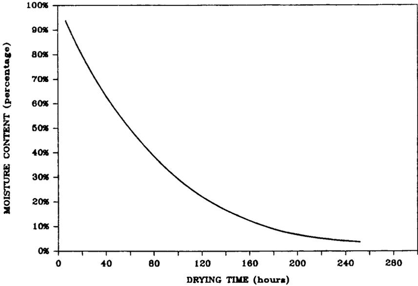
Figure 2. Conventional drying curve
