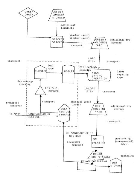
Figure 1. Proposed lumber drying operation
