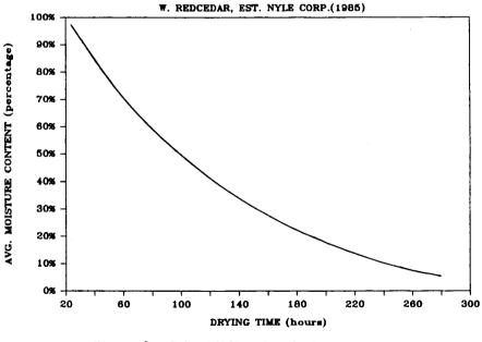
Figure 3. Dehumidification drying curve
