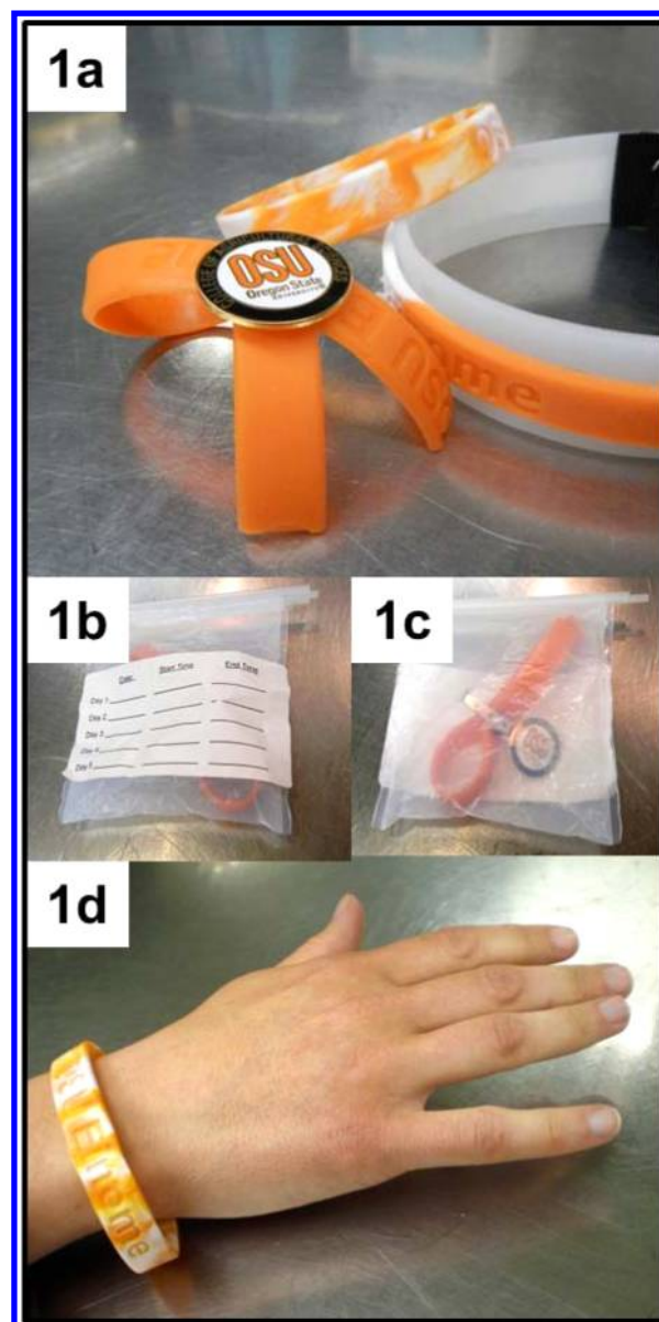
Figure 1. Examples of silicone personal sampling samplers. (a) Configurations of wristbands used in the study including a “single” wristband, one cut and worn as a “lapel”, and as a “stacked” wristband in which only the outer band was analyzed; (b–c) bags used for transport that were attached to track participant ID and exposure time in the occupational deployments; (d) single wristband deployment (debossed writing as pictured: “OSU EINOME”, Oregon State University Environmental Integrated Organic Monitor of Exposure).
