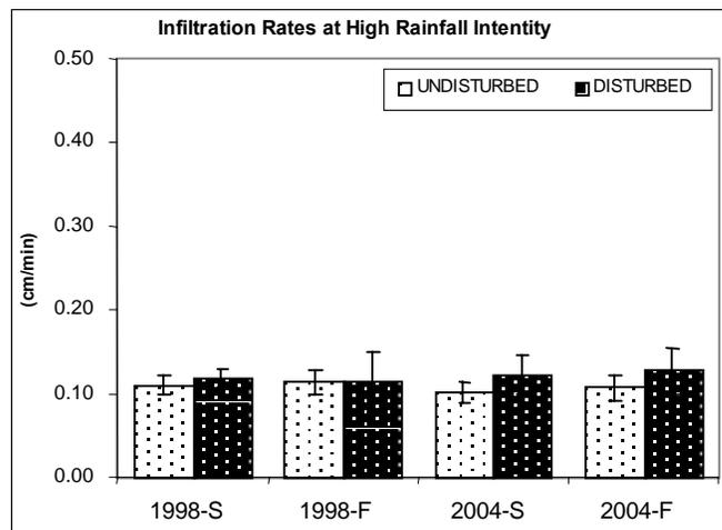
Figure 8. Average infiltration under high rainfall intensity simulations ( $\pm$  one standard deviation).
