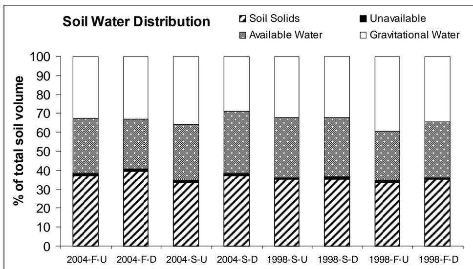
Figure 5. Estimated volumetric distribution of soil solids, available water, gravitational water, and water unavailable to plants based on pressure chamber tests with soil cores.
