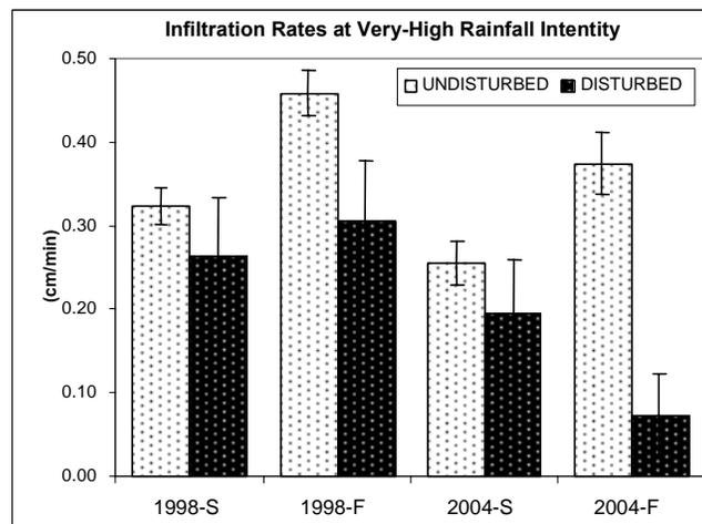
Figure 9. Average infiltration under very-high rainfall intensity simulations ( $\pm$  one standard deviation)
