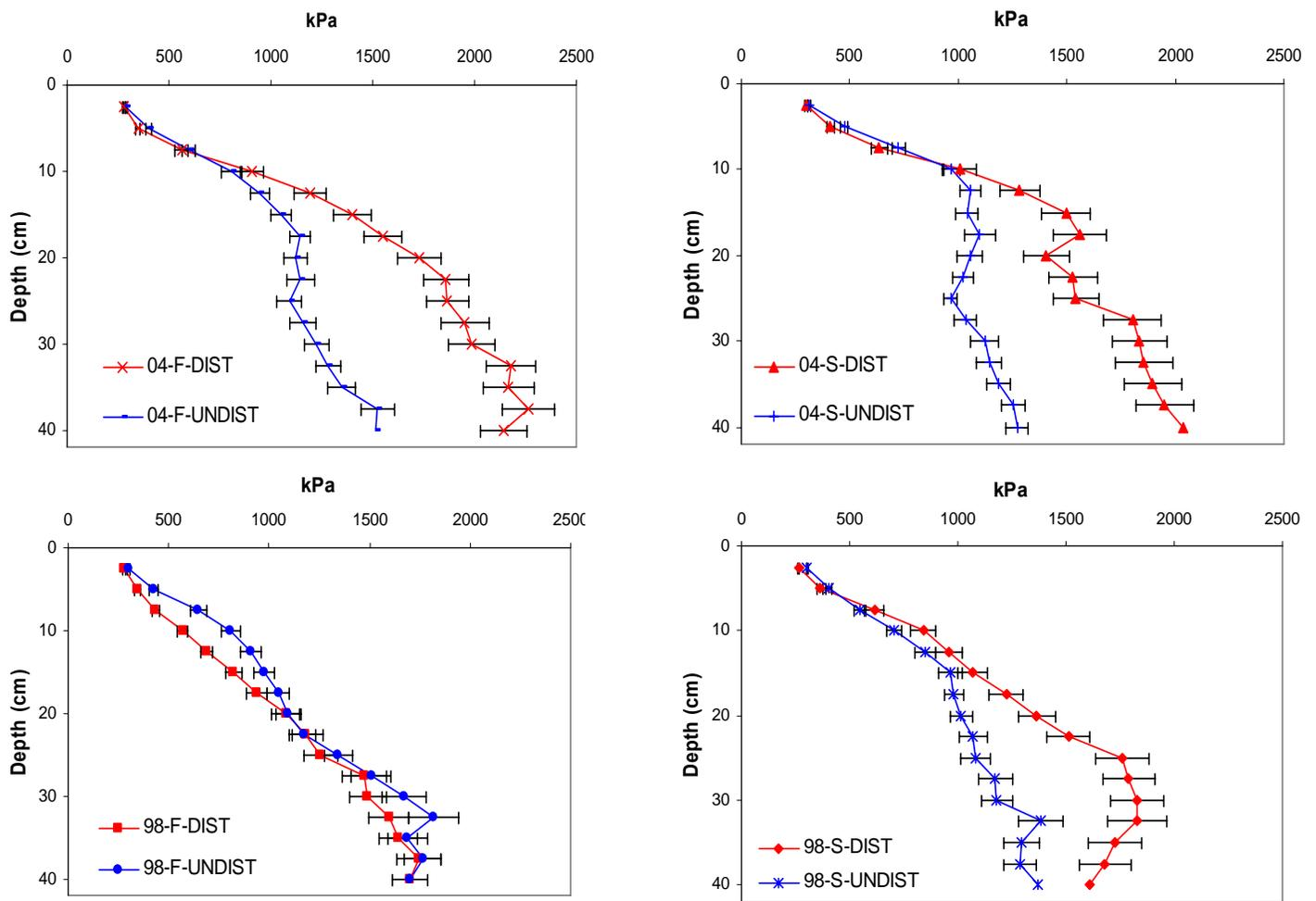
Figure 7: Soil strength by profile type  $\pm$  one standard deviation.
