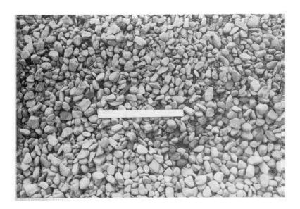
Fig. 8 Sample of the larger size or "drainfield" gravel.
