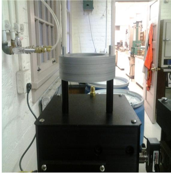
**Figure B.2: Confining rings stacked onto steel rods.**
