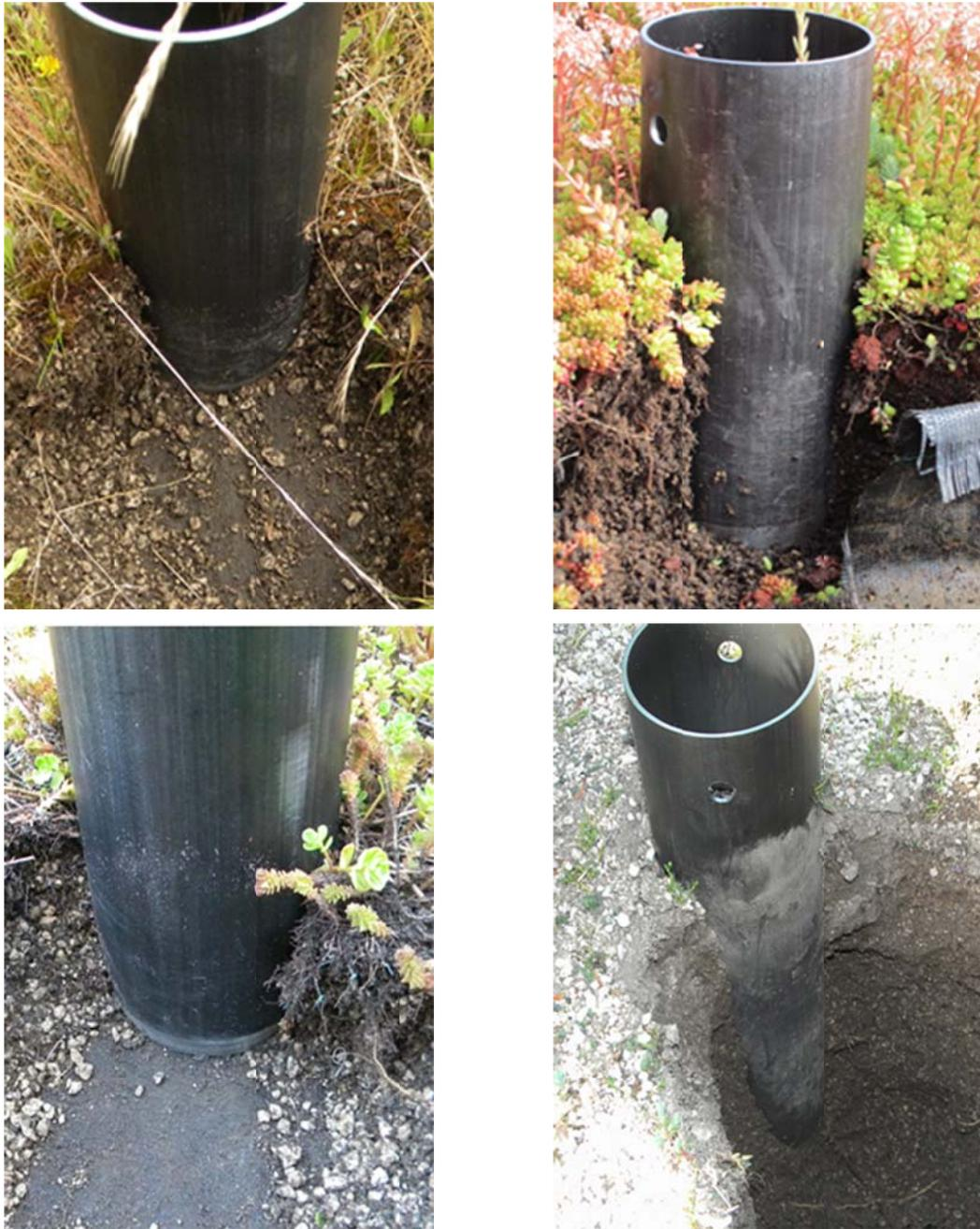
**Figure 1.4: Developed Shelby tube sampler used throughout the field exploration at various encountered ecoroofs. Note the variation in vegetation, soil depth and soil gradation.**
