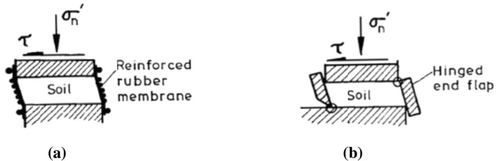
Figure 2.2: Simple shear device developed at (a) NGI (b) Cambridge (after Matthews 1988).
