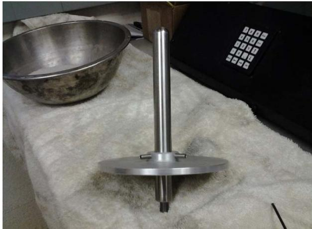
**Figure B.8: Circular plate slid around stainless steel rod.**
