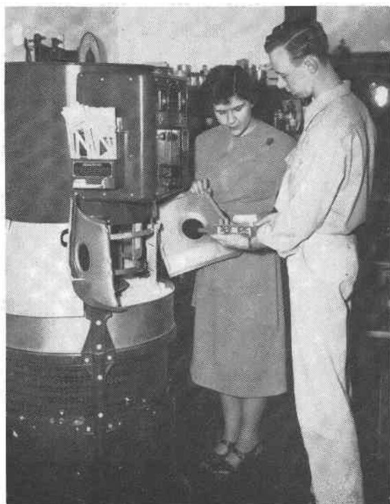
Students in Clothing and Textiles test the light fastness of fabrics in a new machine called the Fade-o-Meter.
