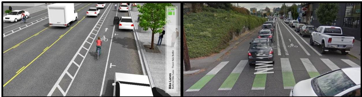
Figure 5.1: Example Design of Buffered Bicycle Lane from NACTO (left) (NACTO, 2011) and a Variation of a Buffered Bicycle Lane in Portland, OR (right) (Google Maps, 2018)
