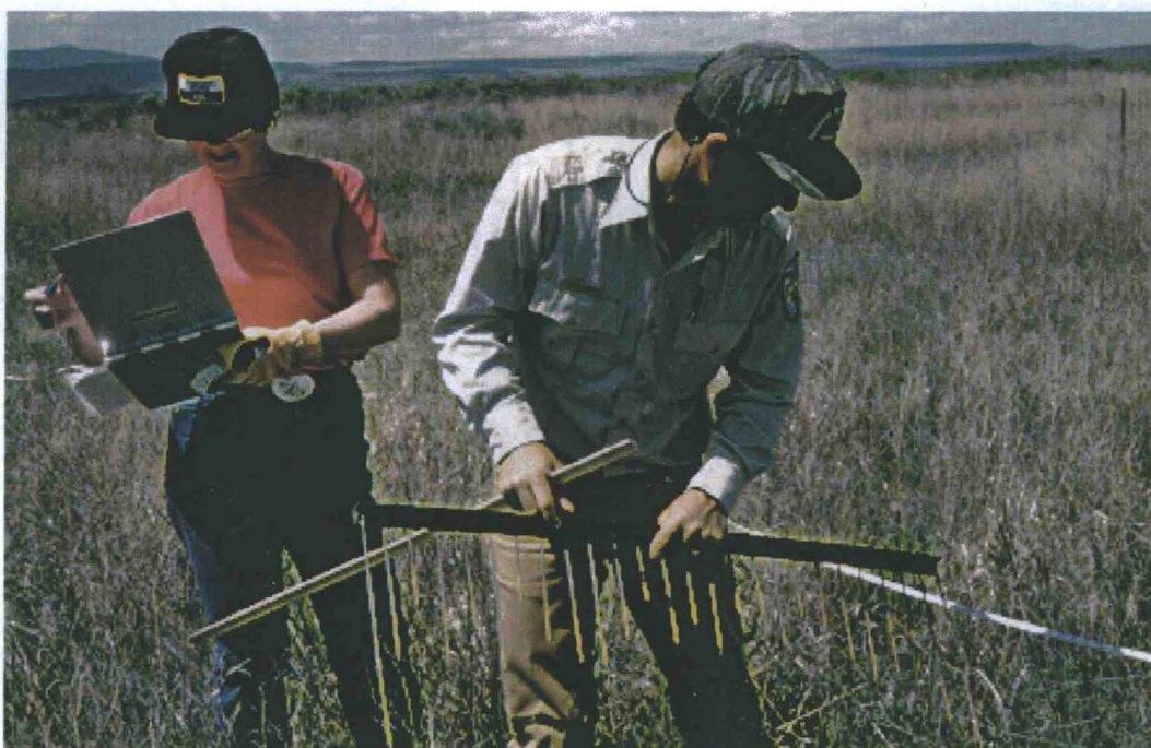
Figure A5. Density and basal cover data were collected along transects using two rectangular 25-point sampling frames.
