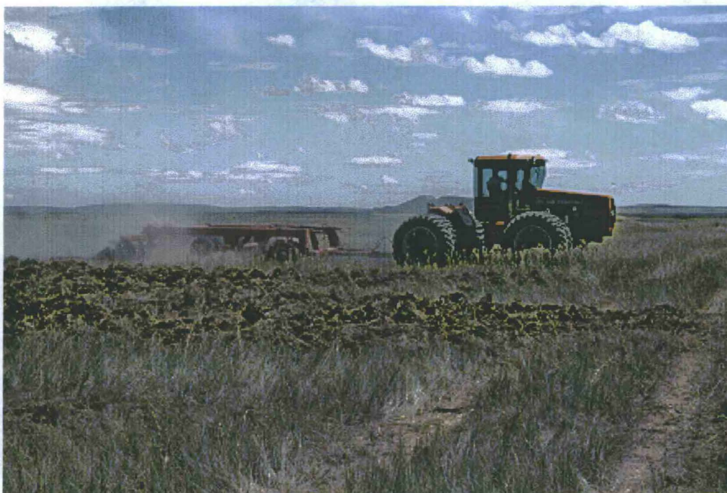
Figure A8. Disking was used to cut, unearth and dry rhizomes in 1995 using a 4.3 m wide disk.
