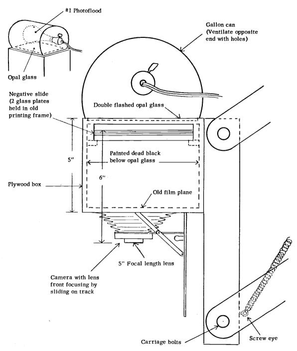
Caution: The bolts holding the two arms to the frame must be precisely the same distance apart as the bolts securing the arms to the enlarger so the enlarger can move up and down vertically.
