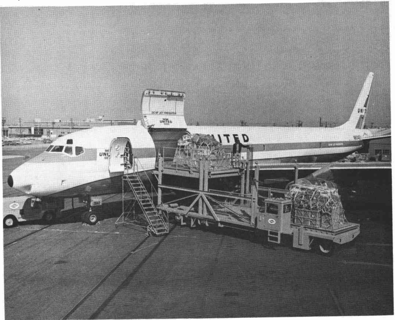
CARGO JET -- Cavernous door on United Air Lines DC-8F Jet Freighter is raised to accept palletized cargo from special Freightair loaders and transporters used at the airline's key cargo cities. Special loading equipment can deliver 13 pallets to plane in 22 minutes.
