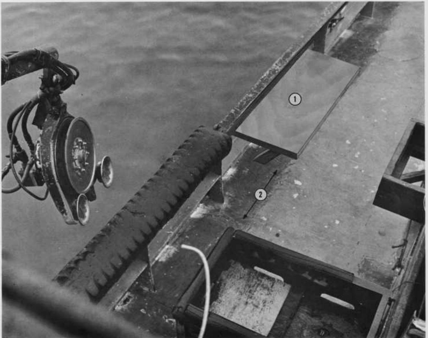
Figure 6. Block rigged for long lining. A folding platform is anchored to the rail as a ready base for pots.
