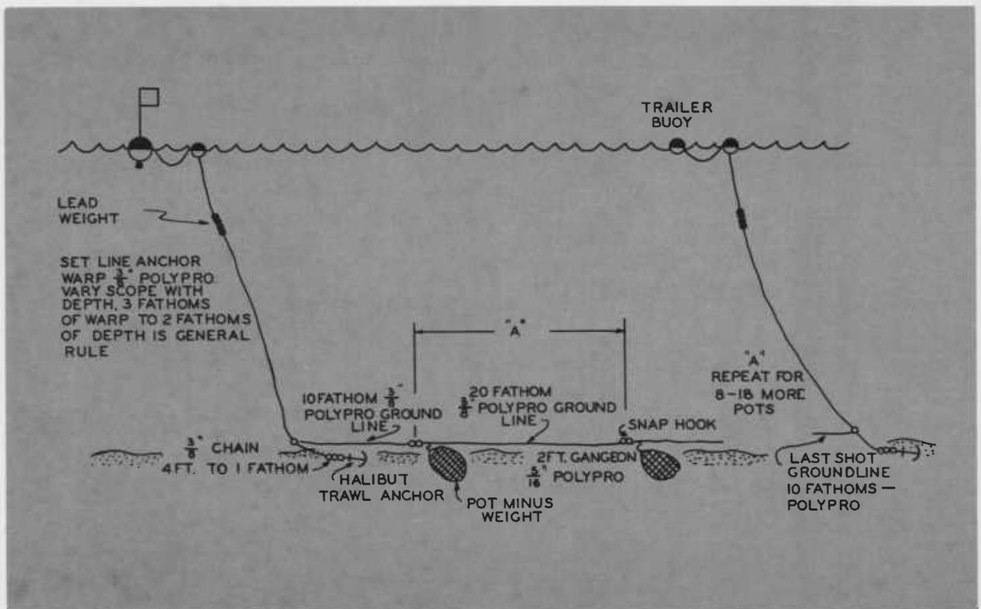
The long-line crab pot system is buoyed and anchored at both ends to keep the string tight and straight. Large buoys and ample scope on the anchor lines will ensure retrieval even in conditions of strong current. Braided or hard-laid polypropylene in 3/8-inch diameter should be used for anchor warps and the ground line and a 3/8-inch swivel should be used between every three to five pots to prevent line kinking. Swivels of larger diameter may slip in the
