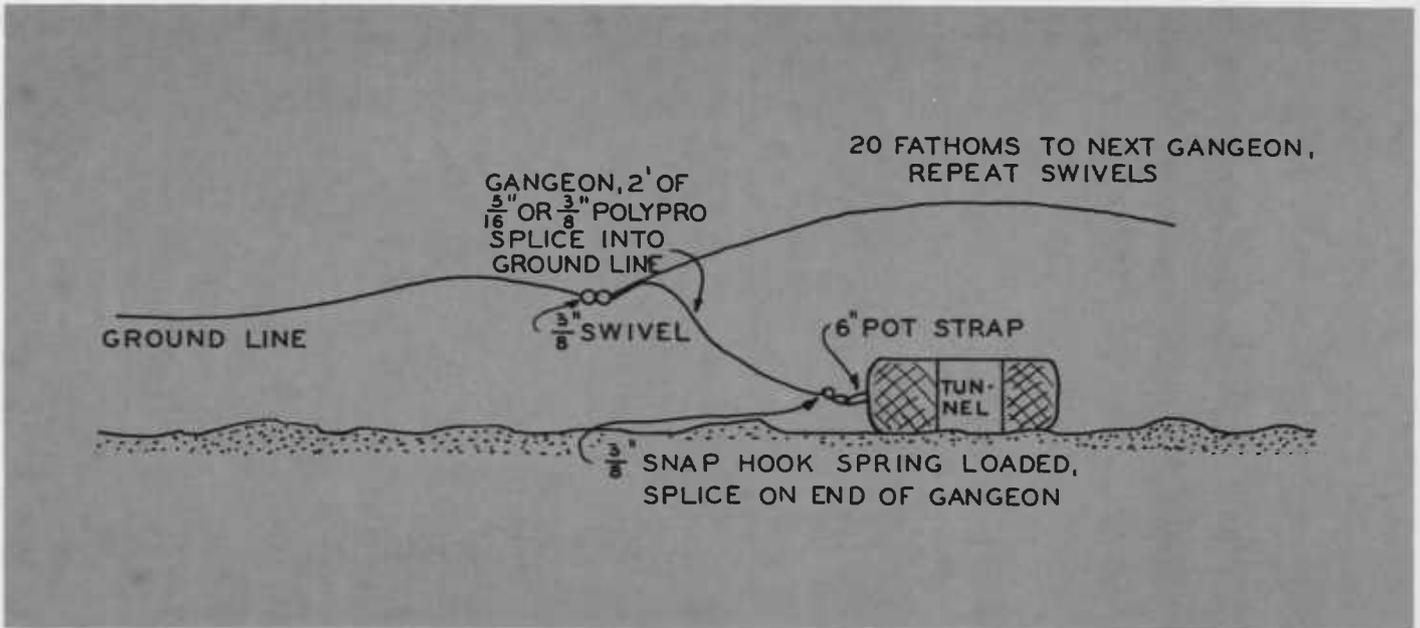
The ground line should run for at least 10 fathoms from the anchor end to the first pot to ensure that the anchor is well away from the boat before the first pot comes up. From the first pot on, the pots should be spaced at least 20 fathoms apart. Experience may dictate longer shots than 20 fathoms, but this appears to be an effective distance to cut down overlapping fishing radius between pots and
