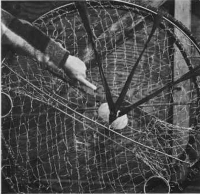
**Figure 5B.** Single-lid cover harness. New longline pots should have lid cover bar made halfway across the top to ease handling with single-lid cover retaining harness.
