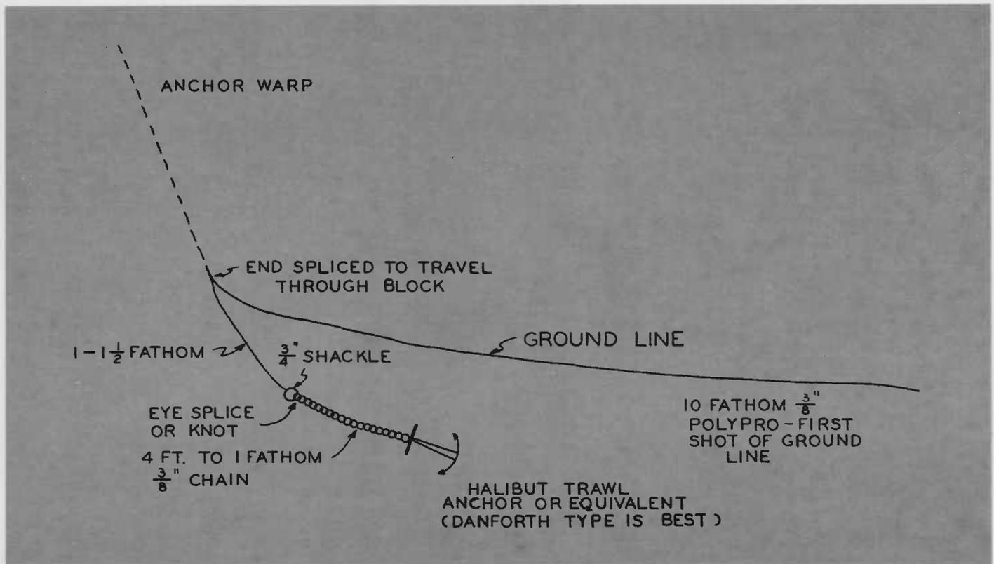
The anchor line should be rigged the same on both ends. A shot of chain is used on the end of the anchor line to ensure positive hold-
