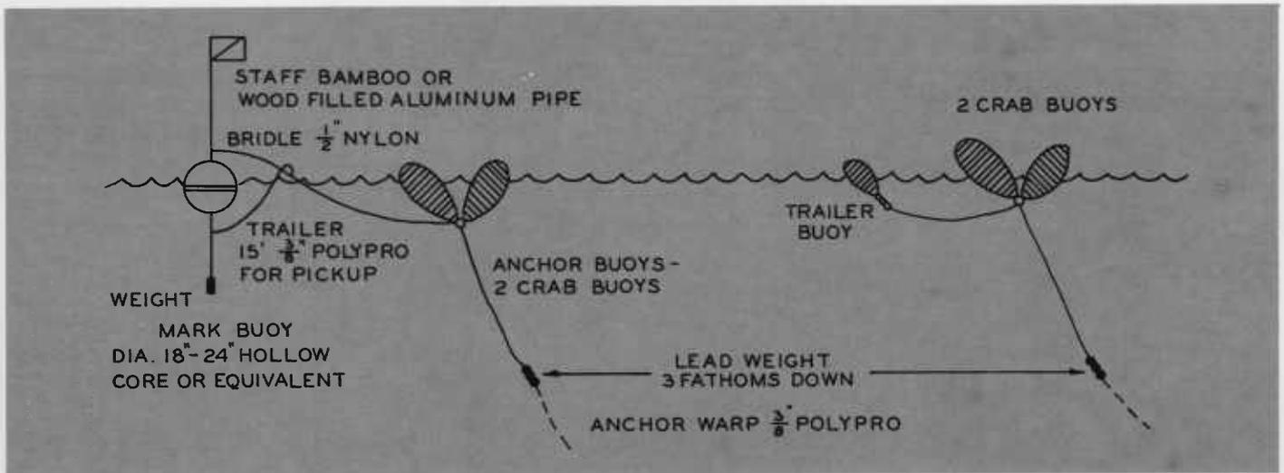
The buoy system used in long-line gear should have enough flotation to allow retrieval in any current conditions. Trailer buoys should be used on both ends to ease grappling and boarding under adverse conditions. Also, buoys at either end mark the spread of
