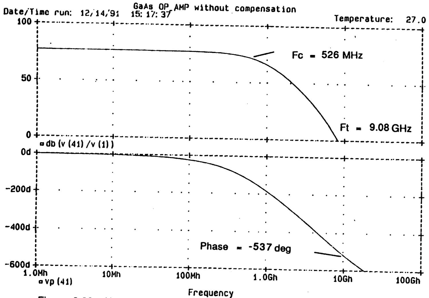
Figure 3.20 Uncompensated composite cascode differential amplifier gain & phase plot
