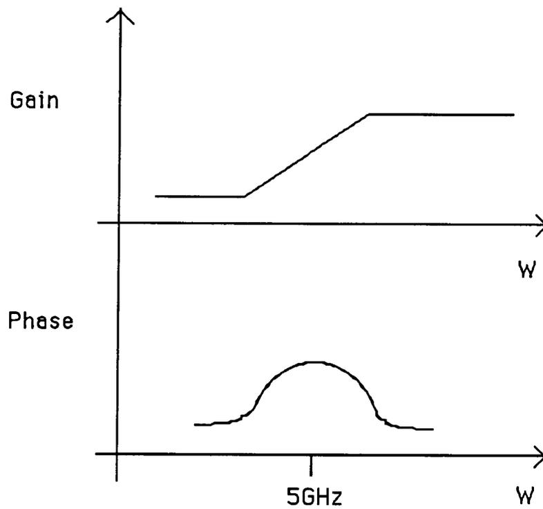
Figure 3.14 Impact of embedded inductor on the phase plot
