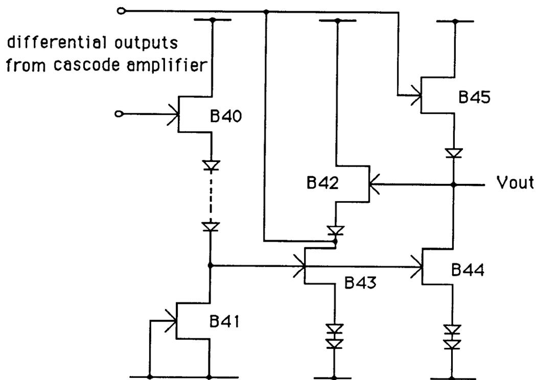
Figure 3.9 Class AB Output Stage
