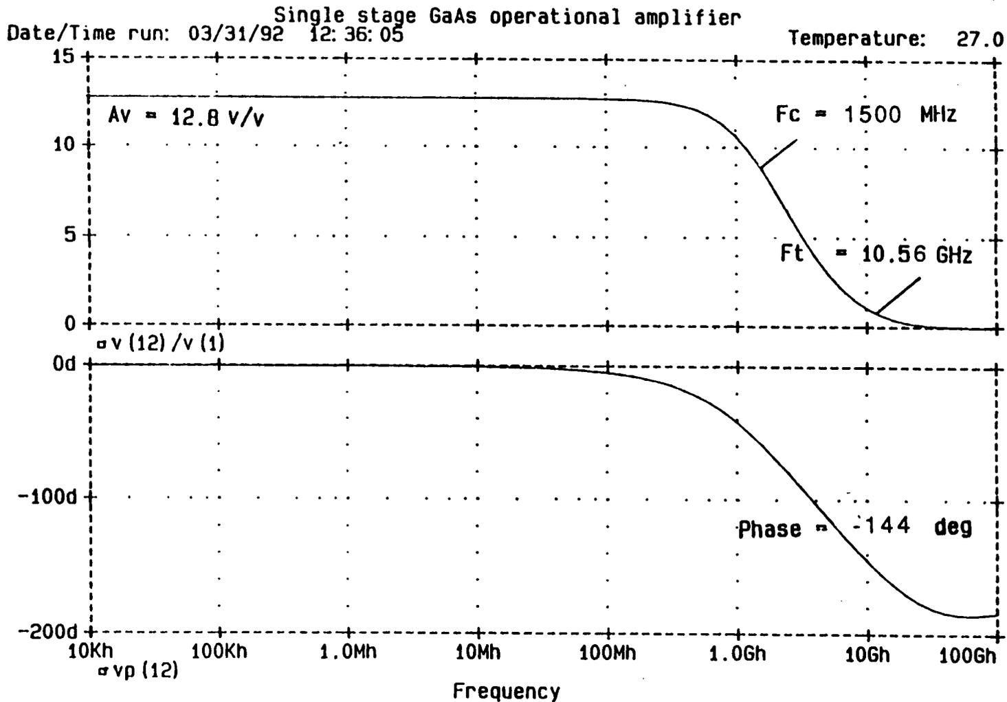
Figure 3.5 Single stage cascode differential amplifier gain & phase plot
