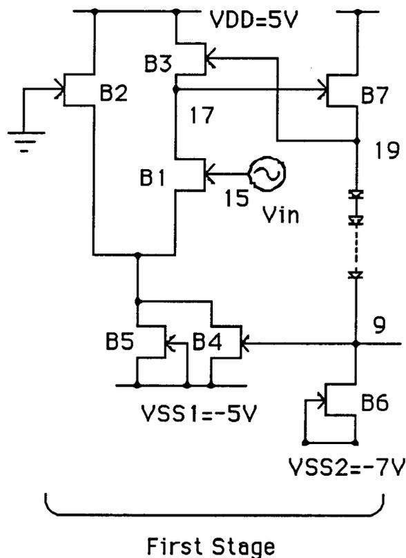
Figure 4.4 First Stage or Differential to Single-ended converter of Toumazou's Composite Operational Amplifier
