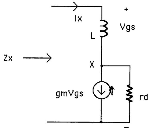
Figure 3.15 AC equivalent circuit of embedded inductor
