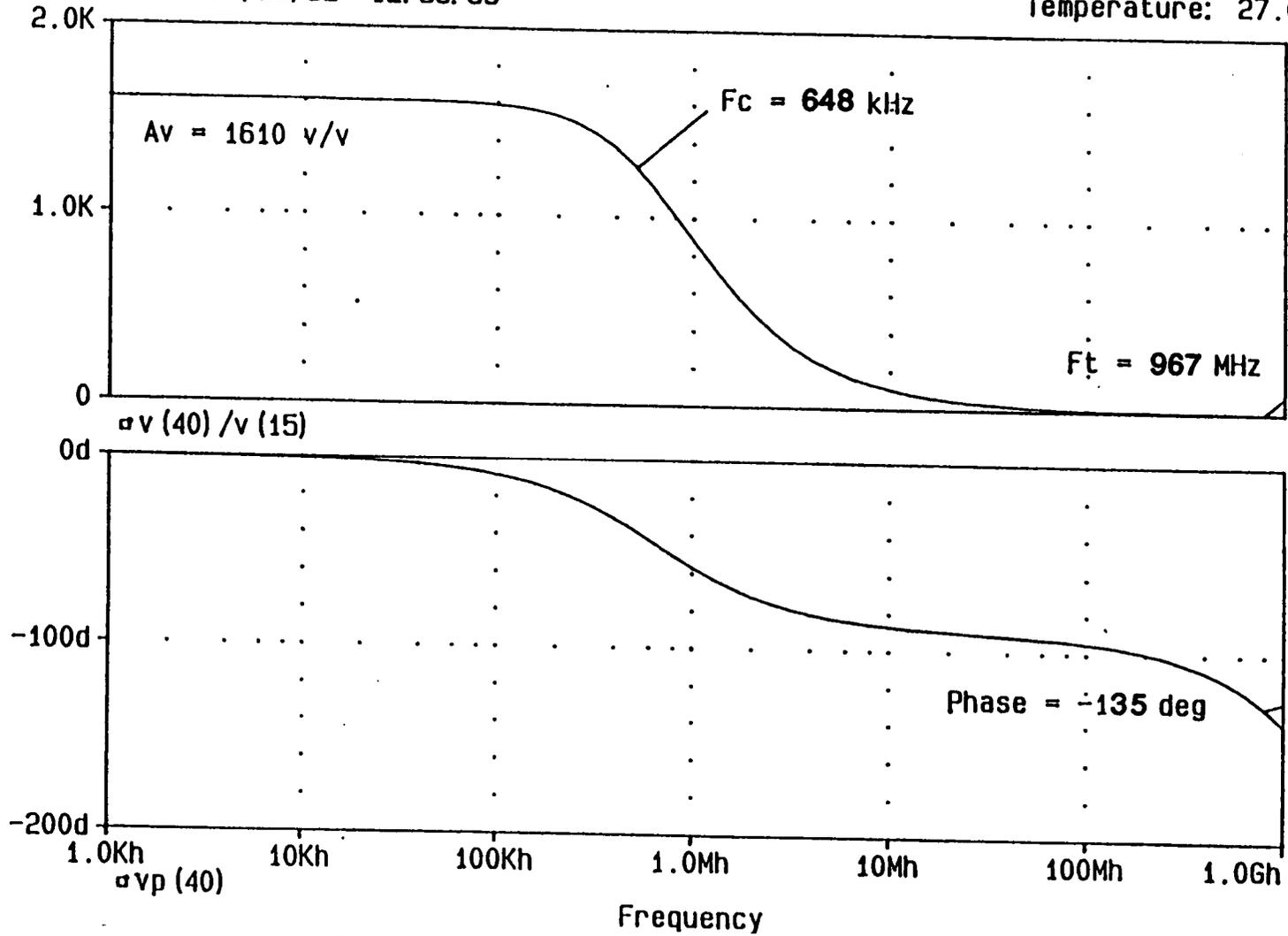
Figure 4.7 Toumazou's circuit gain & phase plot
