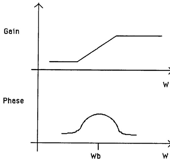
Figure 3.11 Impact of Level Shifter capacitive compensation in the phase plot
