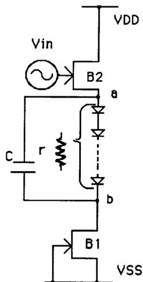
Figure 3.10 Level Shifter capacitive compensation [15]
