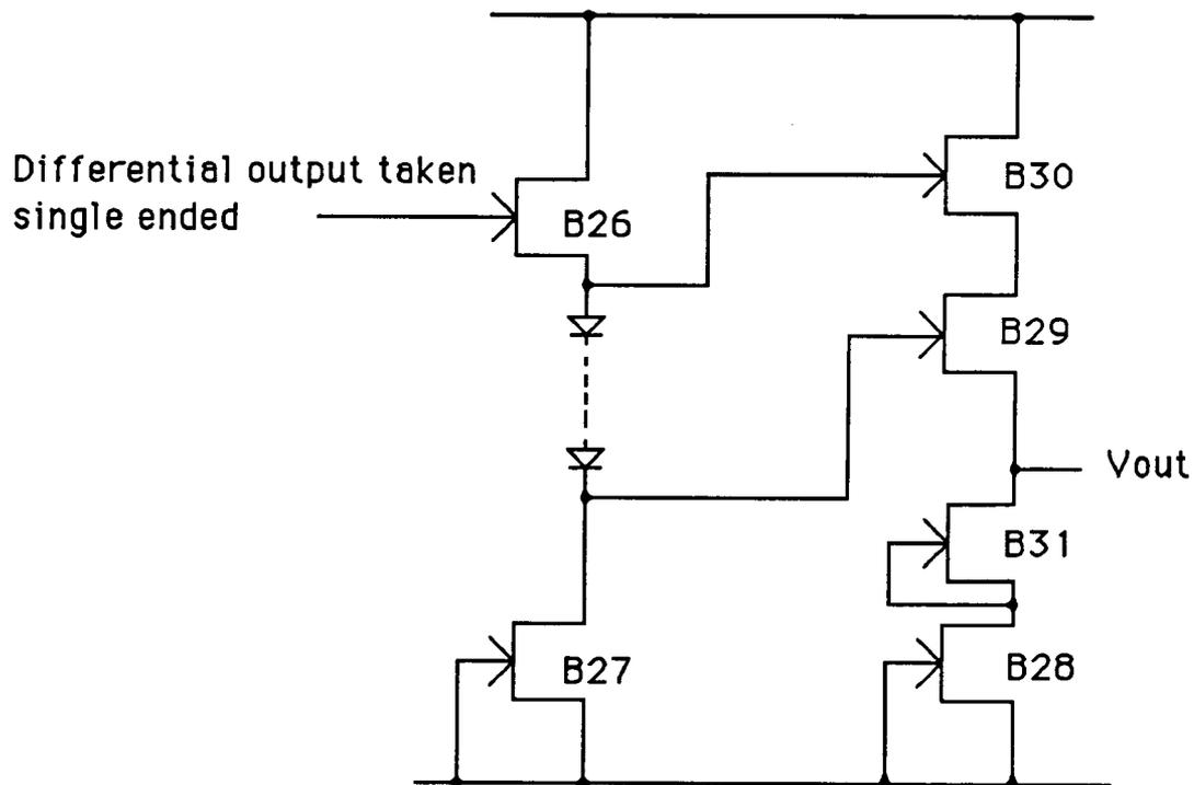
Figure 3.8 Class A Output Stage
