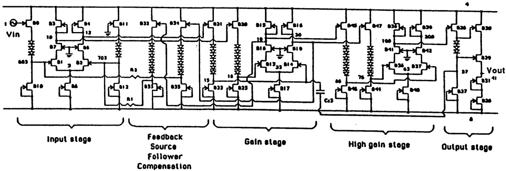
Figure 3.19 Circuit diagram of composite cascode differential amplifier
