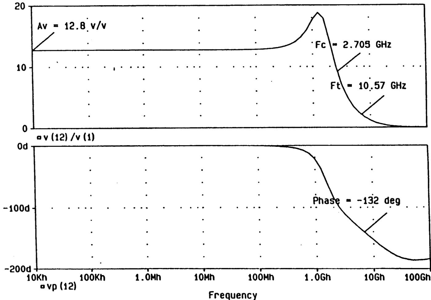
Figure 3.17 Single stage cascode differential amplifier with inductive compensation gain & phase plot
