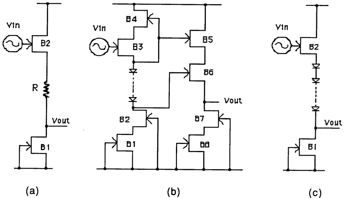
Figure 3.3 Different Level Shifters
