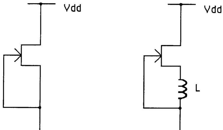
Figure 3.13 Compensation by embedded inductor [16]
