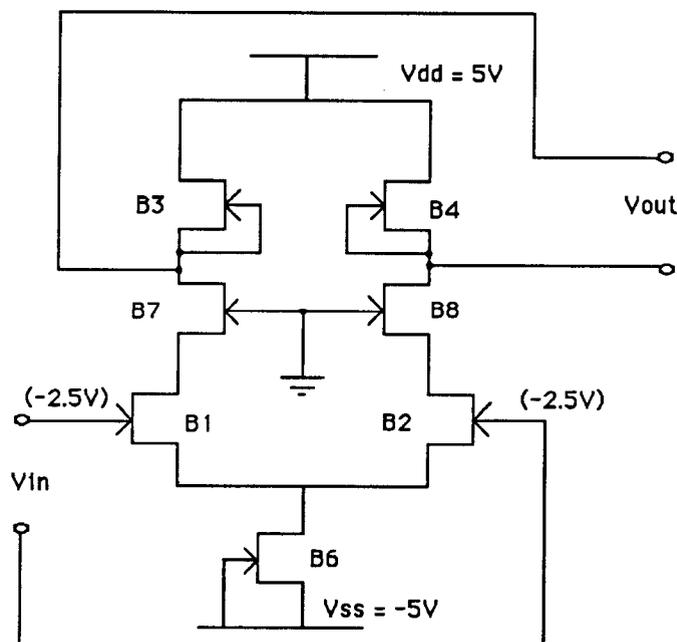
Figure 3.1 Single stage cascode differential amplifier
