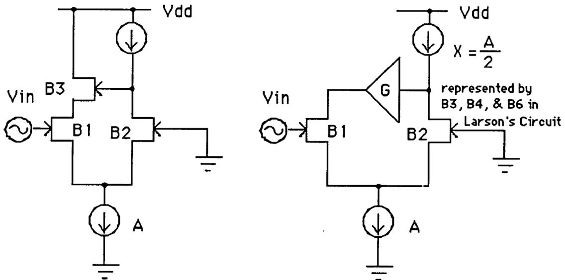
Figure 4.1 Bootstrapped Gain-Enhancement Techniques
