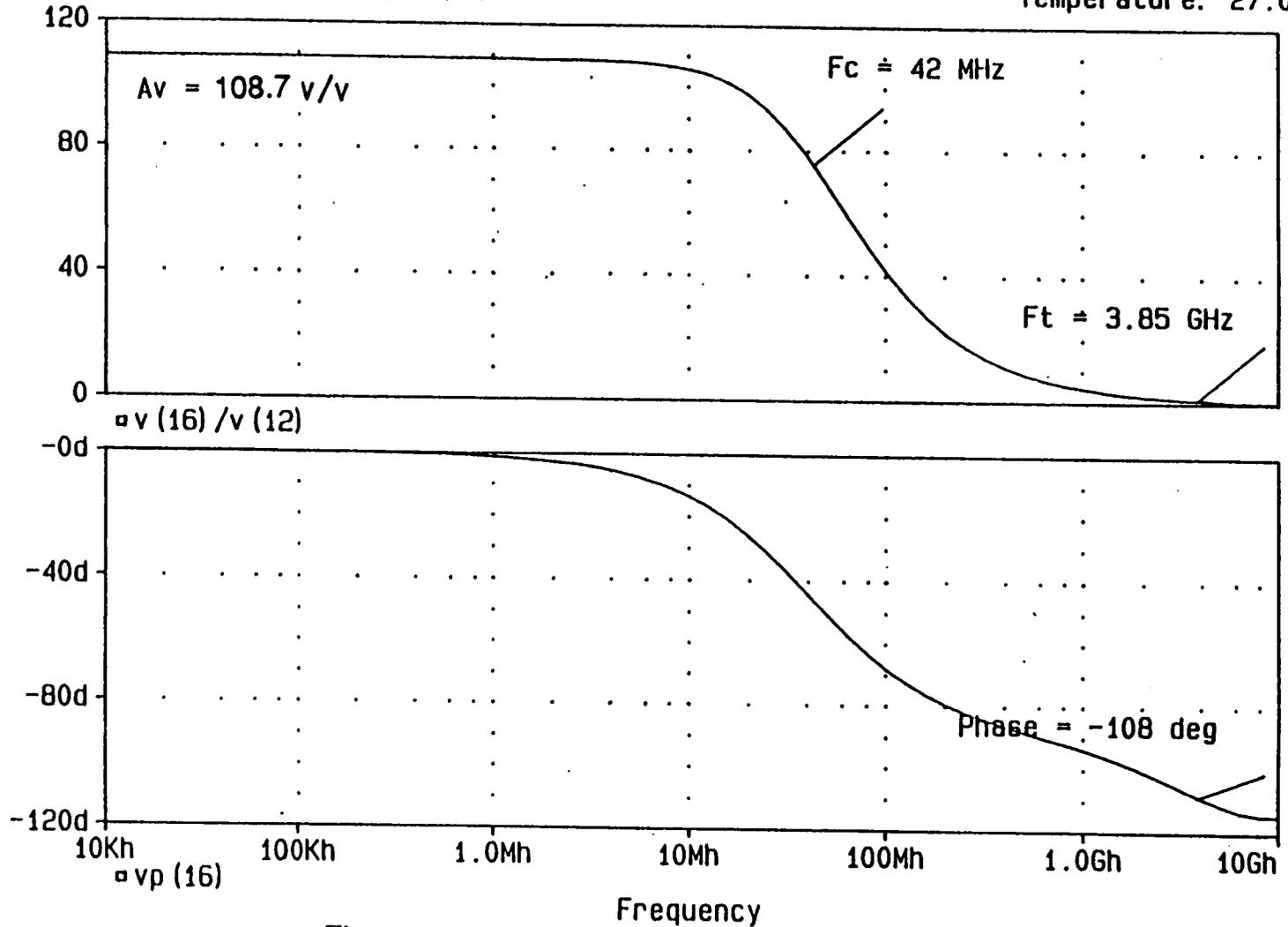
Figure 4.3 Larson's circuit gain & phase plot
