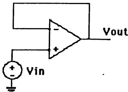
Figure 3.22 Test Circuit for Slew Rate determination
