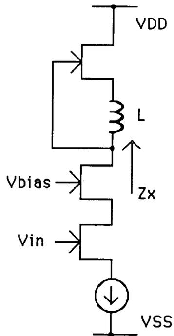
Figure 3.16 Cascode amplifier with inductive compensation
