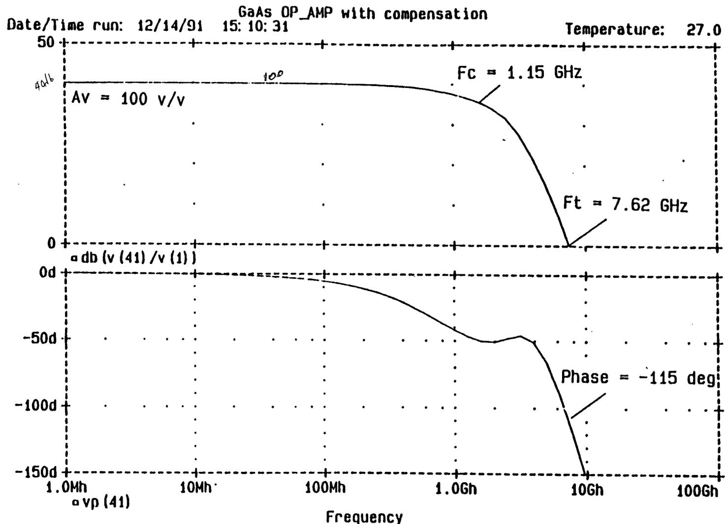
Figure 3.21 Compensated composite cascode differential amplifier gain & phase plot
