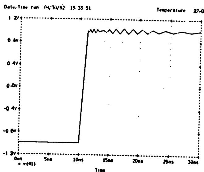
Figure 3.23 Pulse response for +/- 1V step input
