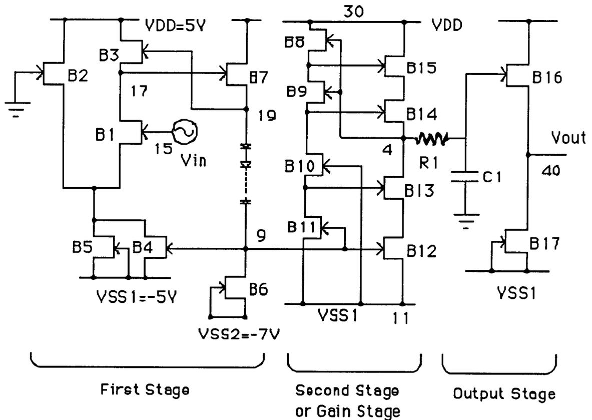
Figure 4.6 Complete Toumazou's Composite Operational Amplifier with Compensation
