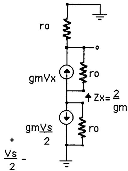
Figure 3.2 AC equivalent half circuit of the cascode differential amplifier
