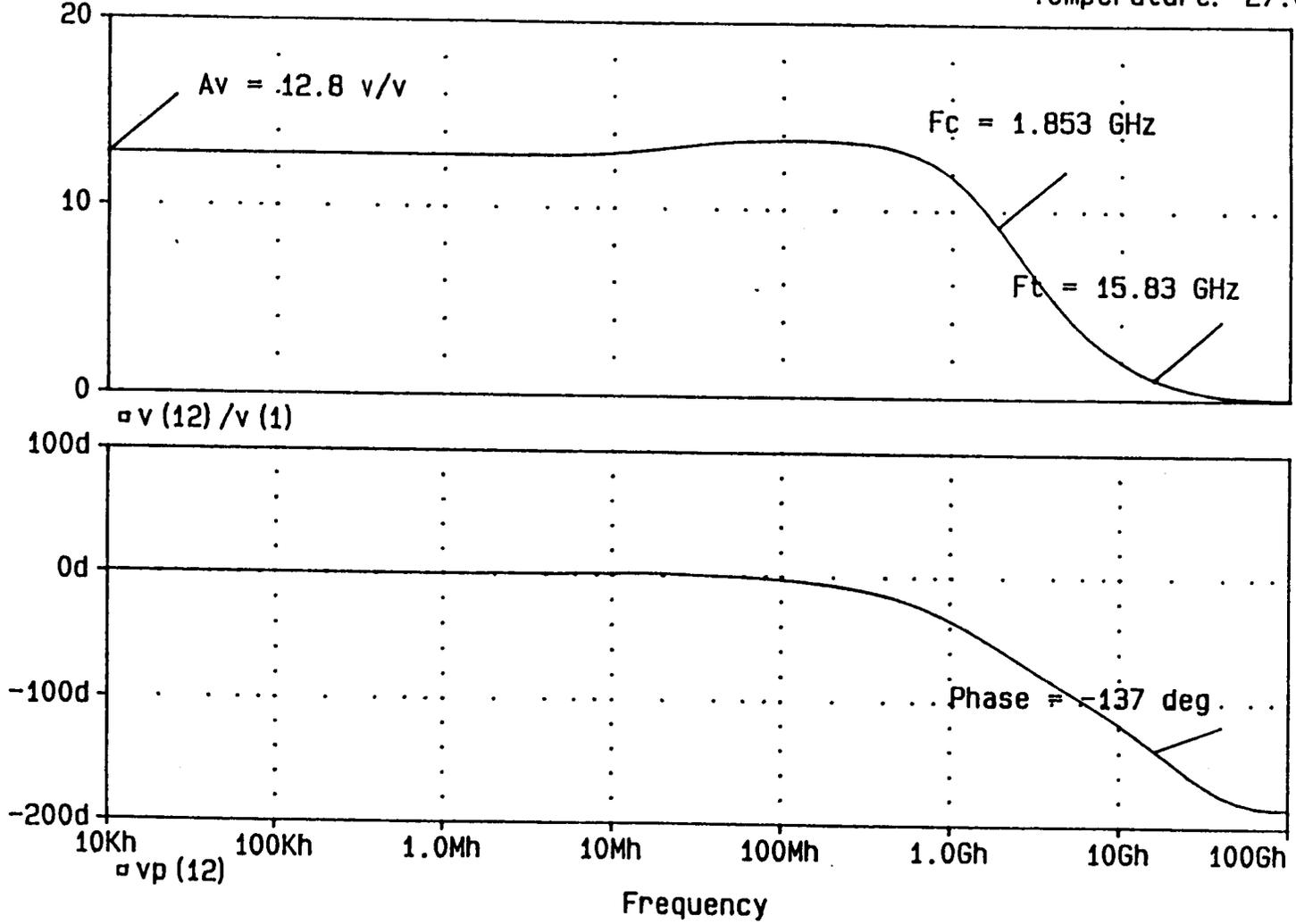
Figure 3.12 Single stage cascode differential amplifier with capacitive compensation gain & phase plot
