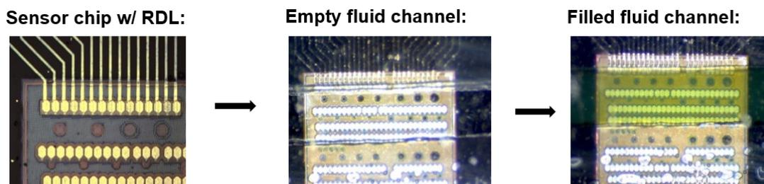
Figure 4.5: Laser-cut microfluidic overlay: (left) Co-planar encapsulated photodiode array IC with FOWLP connections to on-chip pads. (center) Prepared substrate with (empty) laser cut microfluidic channel. (right) Prepared substrate with die filled microfluidic channel.
