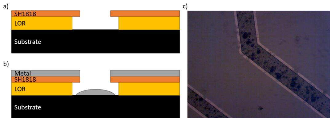
Figure 3.5: Lift-Off-Resist (LOR) process: (a) When SH1818 is developed LOR is also dissolved away faster than the SH1818 leaving an overhang. (b) When metal is sputtered on the surface because the sputtering comes from all directions metal adheres under the overhang. (c) Image of bare epoxy disk with LOR and SH1818 patterned on top. The light area on the edge is the SH1818 overhanging the LOR.
