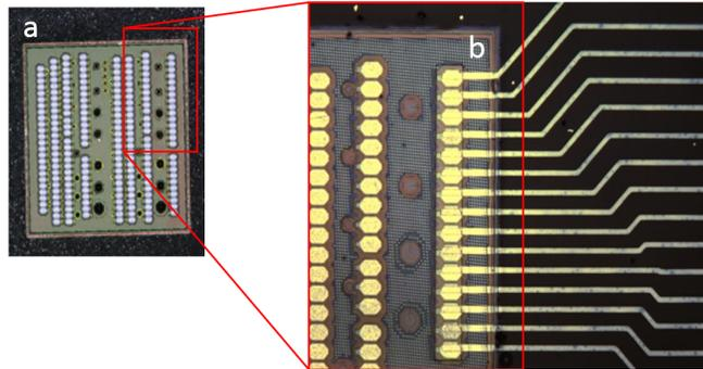
Figure 4.2: Fanout of metallized traces on a CMOS chip array of photo diodes. (a) Image of the bare photodiode array embedded in over-molded epoxy. (b) Traces were taken from both sides of the chip in a FOWLP process. Improved connectivity yield was found in traces from larger continuous openings in the passivation layer.
