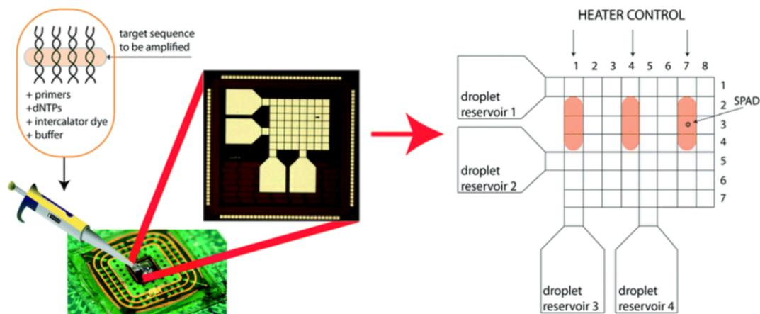
Figure 2.8: Droplets of the test sequence and PCR reagents are delivered to one of four reservoirs on the chip. The entire surface is heated with three heaters at columns 1 4, and 7. Measurements can be made from the photodiode located at (3,7) [27].
