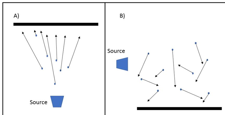
Figure 3.3: Metal deposition: a) Metal evaporation is emitted from a single point forming a monolithic layer of metal. b) In metal sputtering the metal particles approach the substrate from all directions, giving a more even distribution of metal on all surfaces.
