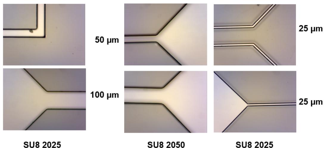
Figure 3.10: Microfluidic channels were fabricated in channel widths ranging from 20 to  $100\ \mu\text{m}$  and heights of 50 or  $100\ \mu\text{m}$  depending on the type of SU-8.
