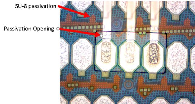
Figure 3.2: SU-8, a clear patternable epoxy, covers the entire surface of the chip with the exception of openings used to access bond pads on the chip.
