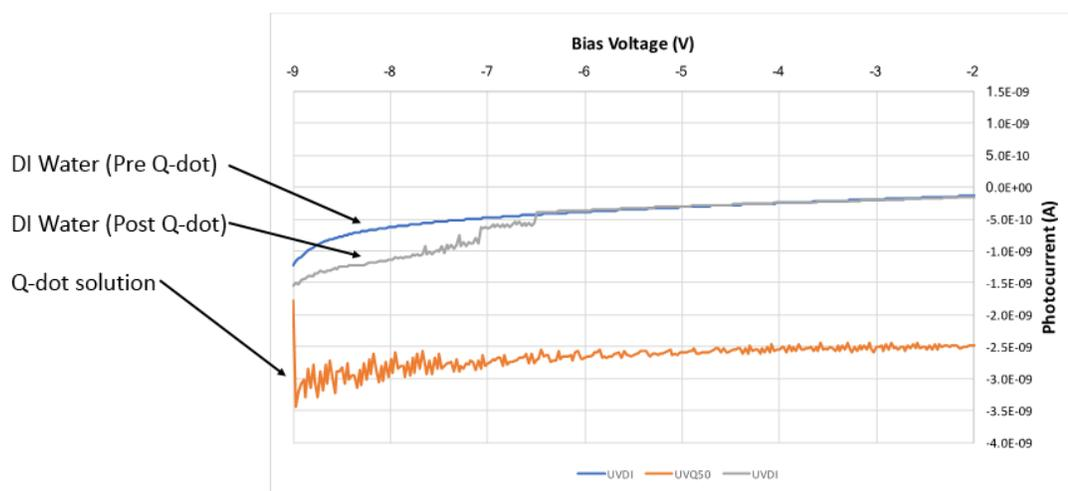
Figure 4.8: Optical detection using quantum dots. An increase of (negative) current was detected when 50% Q-dot solution was passed through the fluidic channels and excited by UV light.
