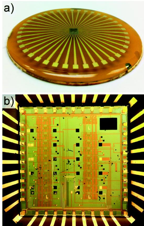
Figure 2.9: CMOS chip encapsulated in epoxy [3]: a) The die is connected to external pads in an Epoxy Molded Chip Carrier. b) close up view of the die and the connections along the chip-substrate interface.
