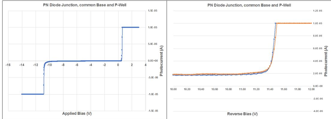
Figure 4.4: Bias measurements made to multi-chip photodiode chips (a) Bias measurement made on individually connected photodiode. (b) Reverse bias measurement of diodes with common bases and P-wells.
