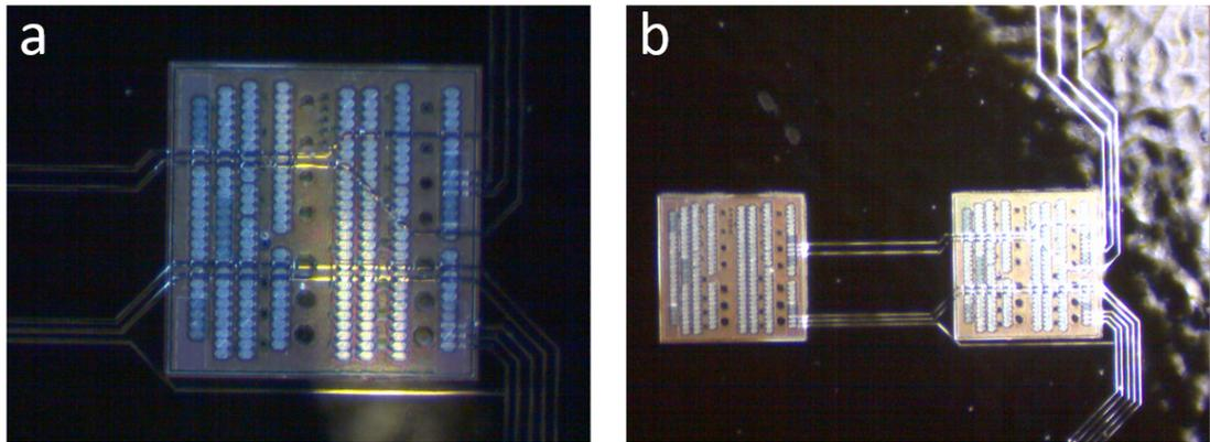
Figure 4.3: Two chips embedded in epoxy substrate. Four diodes, two from each chip, are traced out. (a) The metal traces go across the chip on top of the SU-8 passivation, so as not to interfere with any other part of the chip. (b) The traces start on one chip travel across the second then move away from the chip to probe points.
