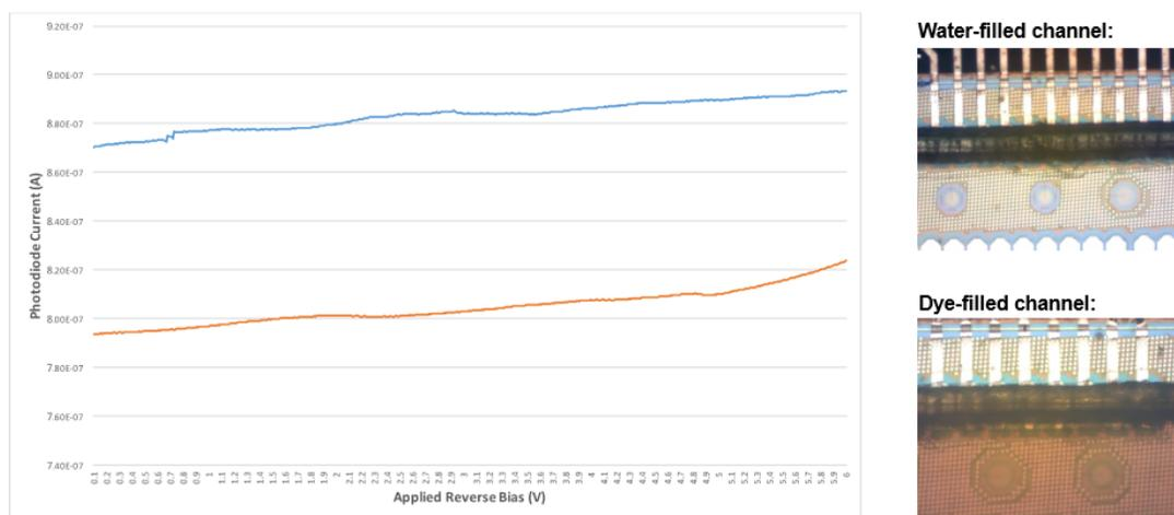
Figure 4.6: Measured IC photodiode current when illuminated through clear and tinted liquids under high illumination.
