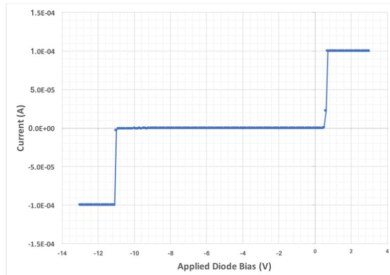
Figure 4.1: The photodiodes were found to have the forward and reverse bias curves at the same voltages as a chip that was not embedded in an epoxy wafer.
