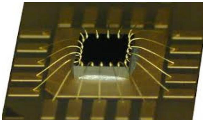
Figure 1.1: Wire bonds are a means of connecting an integrated chip to an external carrier. Wire bonds extrude vertically from the chip and are extremely fragile.
