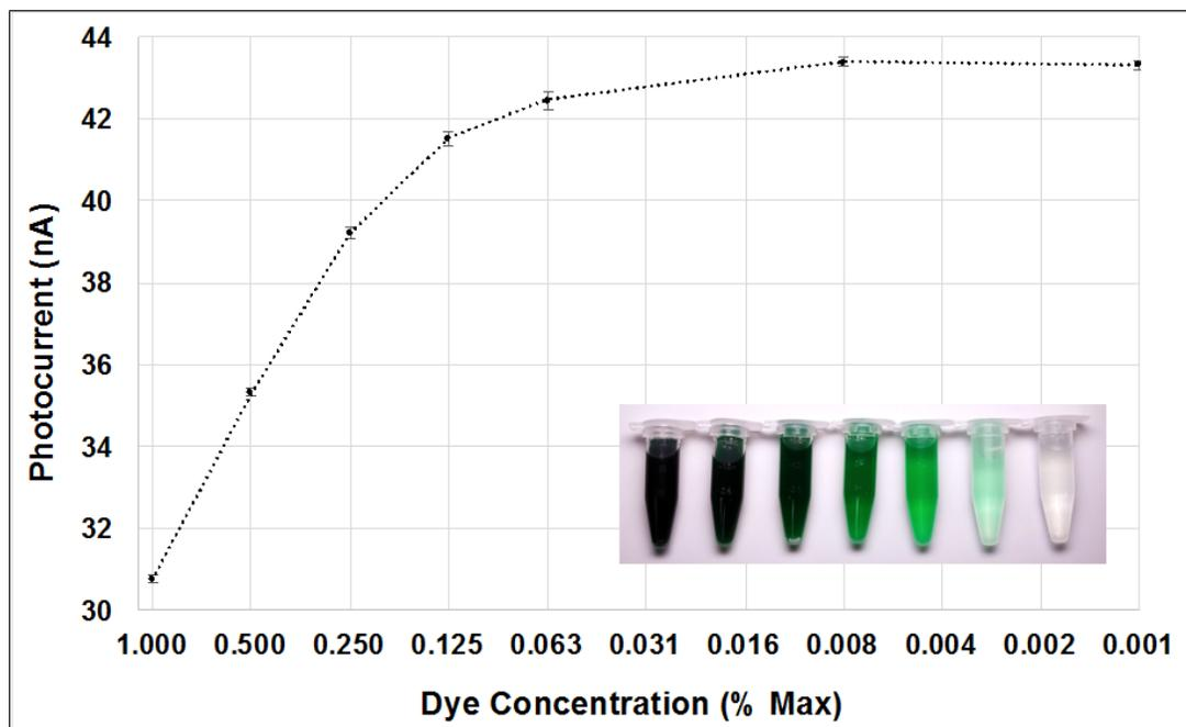
Figure 4.7: Measured IC photocurrent using a serial dilution series to measure optical transmission across a broad range of opacity for use in chromogenic immunoassays.
