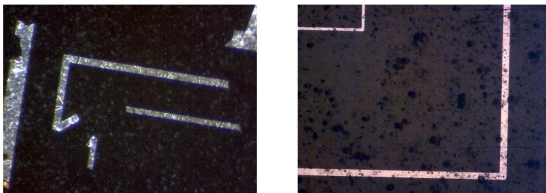
Figure 3.7: Early metal adhesion tests: (left) Metal tended to peel away before we used lift-off-resist in our photo-lithography process. (right) After using LOR, the traces were well defined but the topography and surface roughness of the epoxy caused challenges for connectivity.
