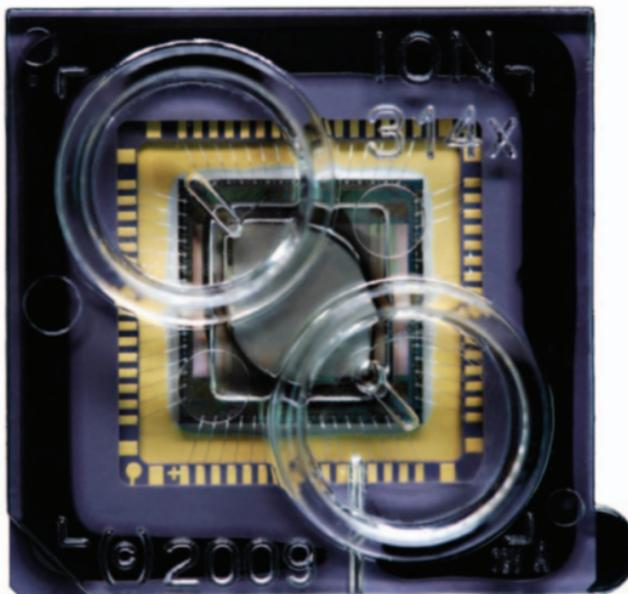
Figure 2.3: A polycarbonate cover to protect the wire-bonds and other electronic parts from the liquid that needs to get to the ISFET sensors in the center of the die. [17]
