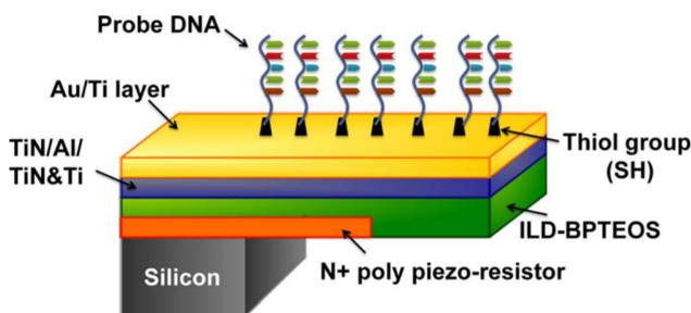
Figure 2.1: Cross-sectional view of micro-cantilever based piezo-resistor for the detection of DNA [19].
