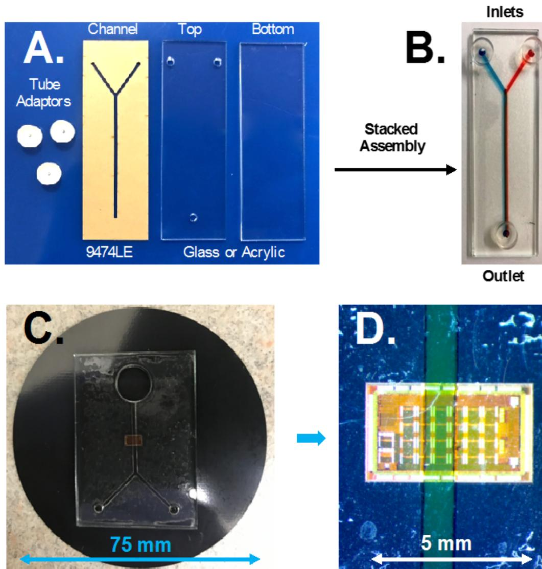
Figure 3.9: Laser-cut adhesive tapes and acrylic sheets (a) are aligned to form laminated fluidic devices. (b) By using a bare IC embedded in an EMC wafer using FOWLP as the bottom substrate, a channel can be rapidly fabricated above a sensor IC for fluid delivery to the chip (c-d).
