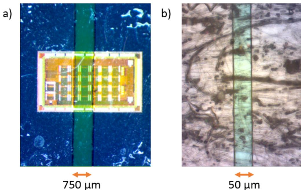
Figure 3.8: Size comparison of microfluidic channels: (A) Laser cut channels are fast and fast to produce, the narrowest channels are 750  $\mu\text{m}$  wide and 170  $\mu\text{m}$  tall. (B) Microfluidics created in SU-8 have been as small as 20  $\mu\text{m}$  but the adhesive cover is not optically transparent.
