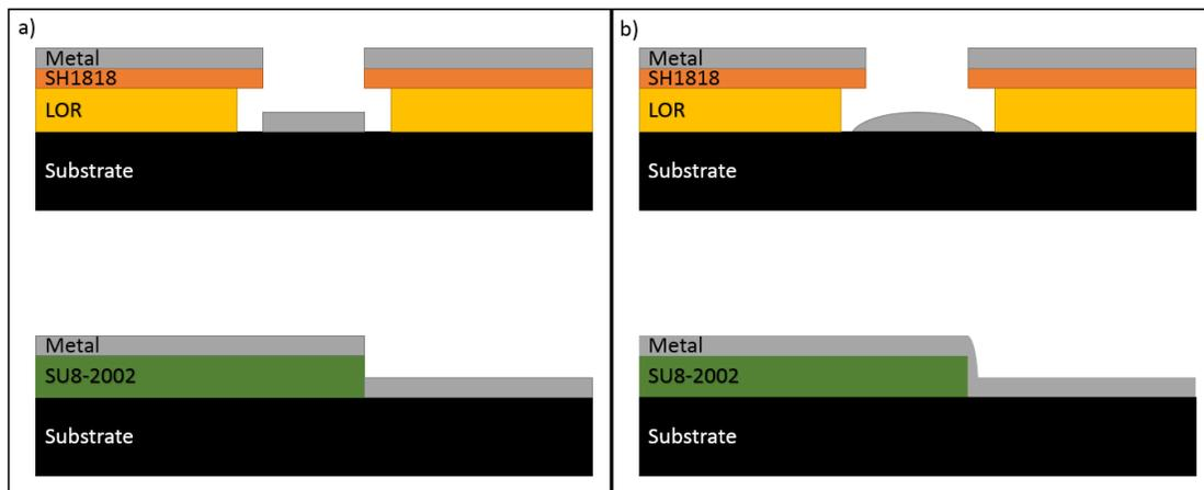
Figure 3.6: Difference between thermal metal evaporation and sputter deposition: (a) In thermal metal evaporation the metal comes from one direction (directly above) which can cause discontinuities. (b) Sputtered metal comes in from every direction, which improves connectivity.
