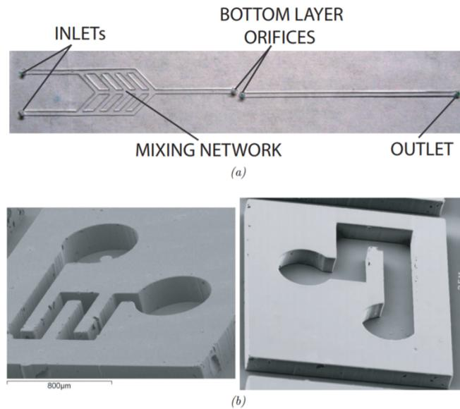
Figure 2.5: To avoid the wire-bonds and other electrical components a multilayered fluidic network is used [24]. a) The top layer contains the inlets, outlet, a mixing network, and orifices that connect to the lower layer. b) Two examples of lower layer networks, the whole of which is smaller than the silicon die.
