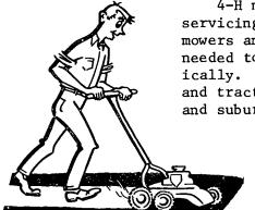
4-H members learn how gasoline engines operate by servicing, operating, and in some cases, repairing lawn mowers and other small engines. Members acquire skills needed to operate engines and equipment safely and economically. It prepares boys and girls for the automotive and tractor projects and is especially suitable for urban and suburban boys.
