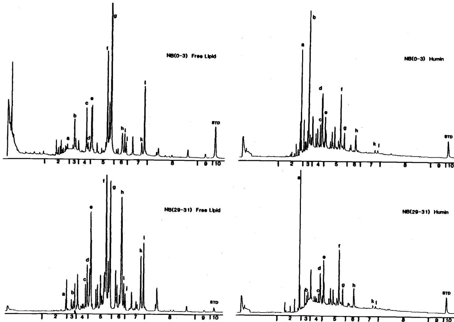
Figure 11. Capillary GC-ECD chromatograms of FL and HU fractions of samples NB(0-3) and NB(29-31). Peak a - pentachlorophenol (methyl ether); other labelled peaks are PCB's. STD - co-injection standard, decachlorobiphenyl.
