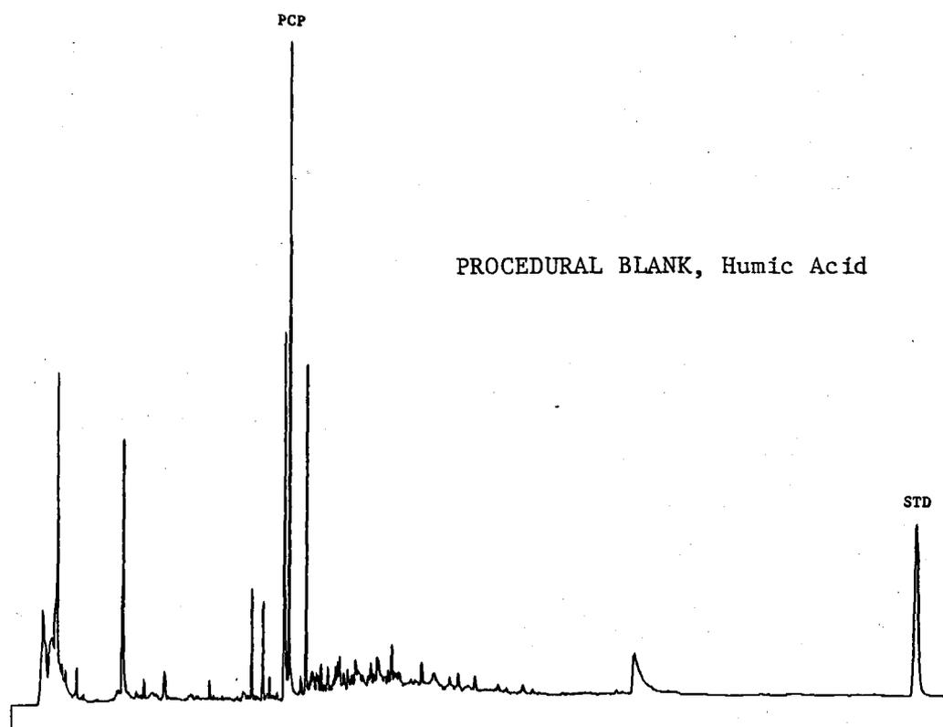
Figure 1A. GC-ECD chromatogram of procedural blank, Humic Acid
