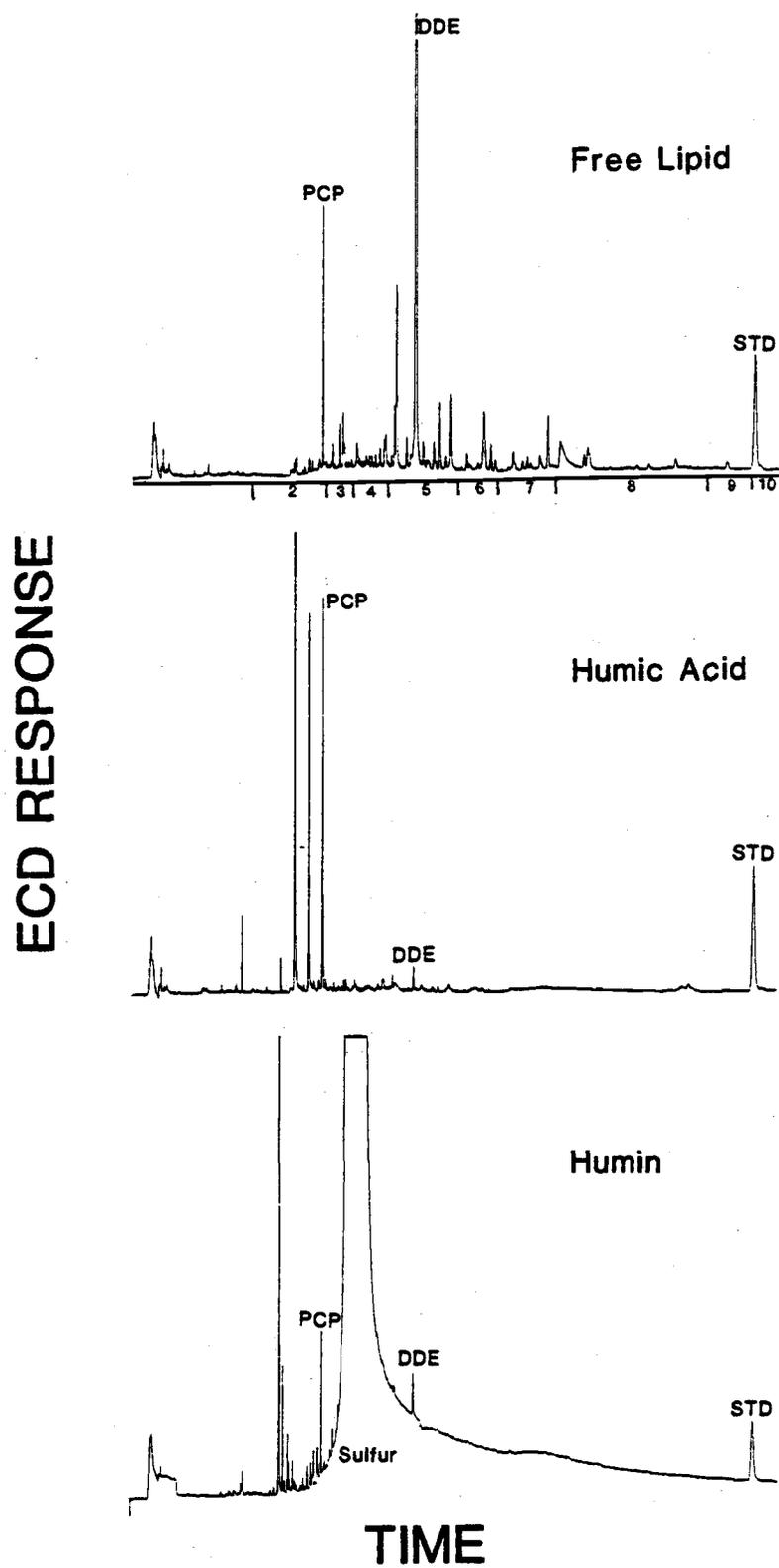
Figure 12. Capillary GC-ECD chromatograms of FL, HA, and HU fractions of sample LA. See legend of Figure 8.
