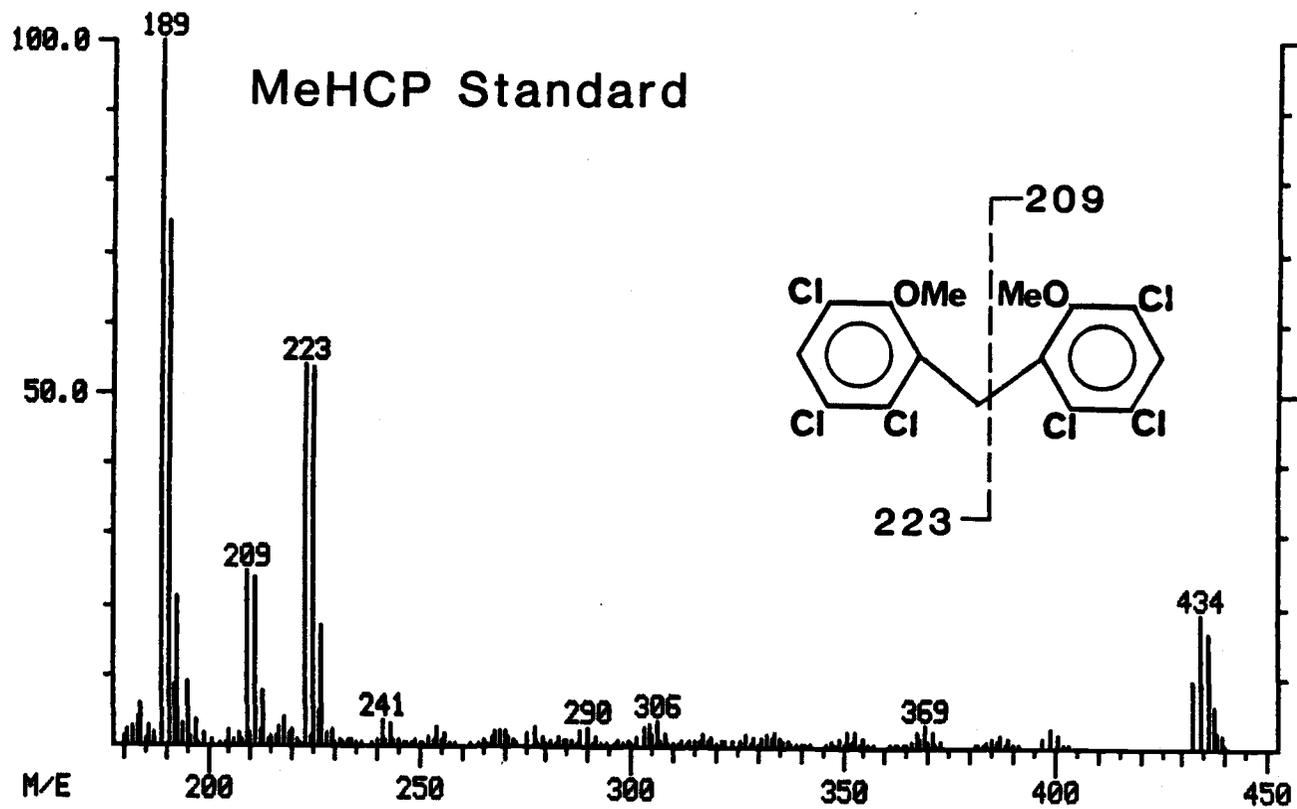
Figure 25. 70 eV mass spectrum of hexachlorophene (dimethyl ether derivative).
