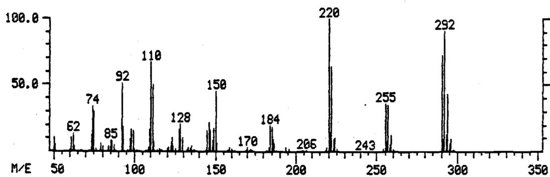
Figure 5. 70 eV mass spectrum of a tetrachlorobiphenyl
