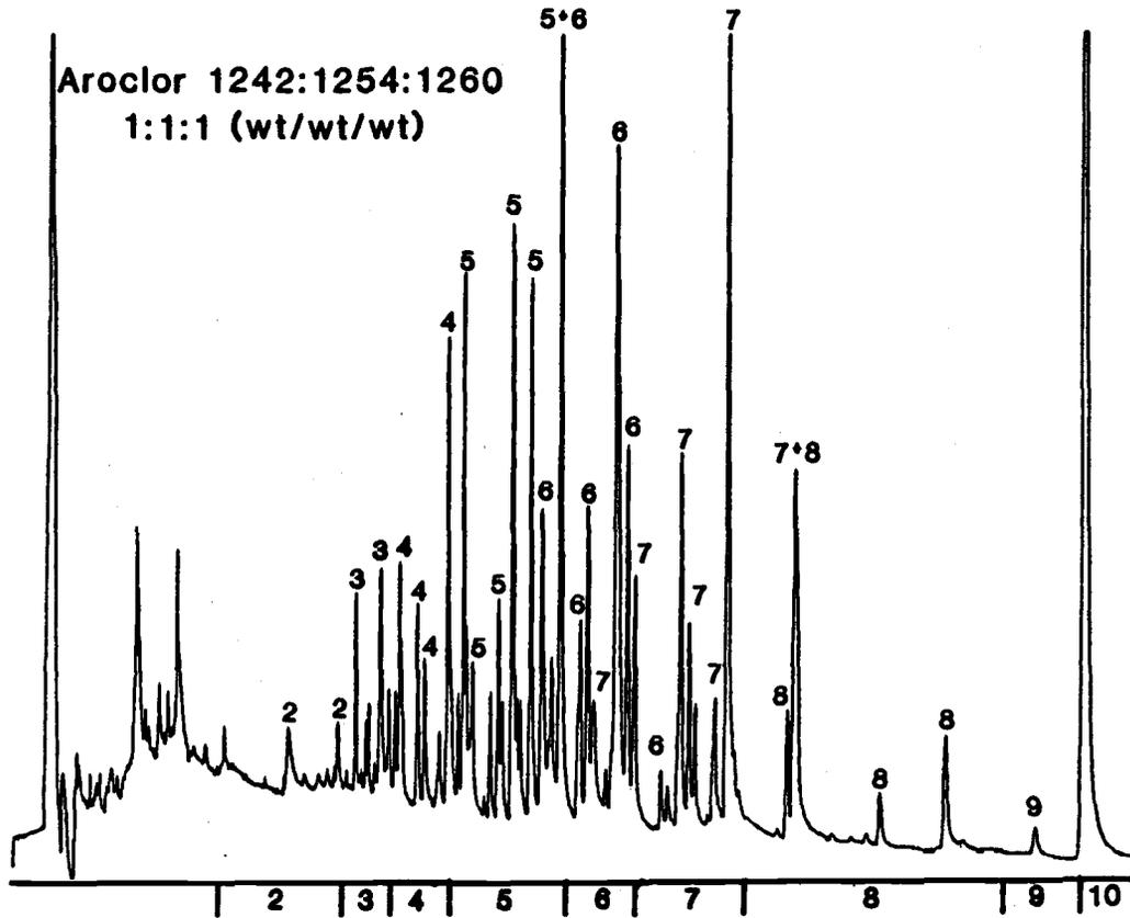
Figure 3. Capillary GC-ECD chromatogram of Aroclor 1242:1254:1260 standard. Approximate elution ranges of PCB homologs are delineated; numbering represents number of chlorine substituents.
