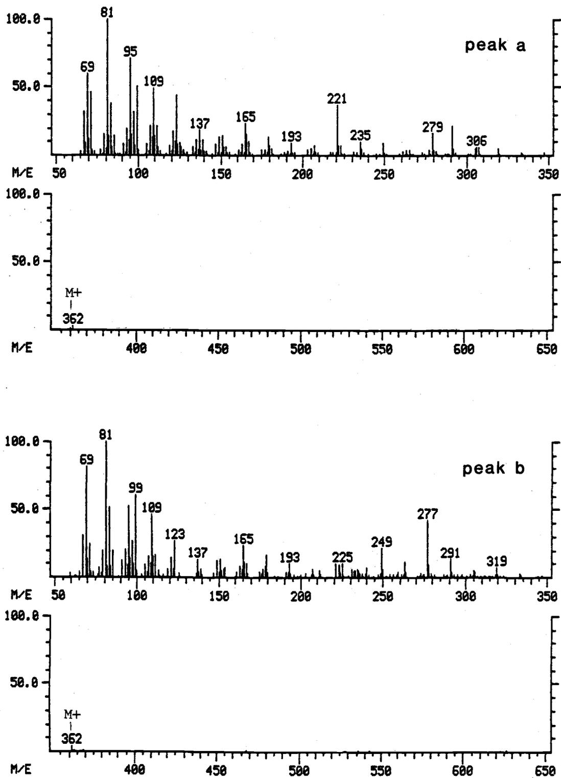
Figure 19. 70 eV mass spectra of peaks a and b in Figure 18, NB(0-3)
