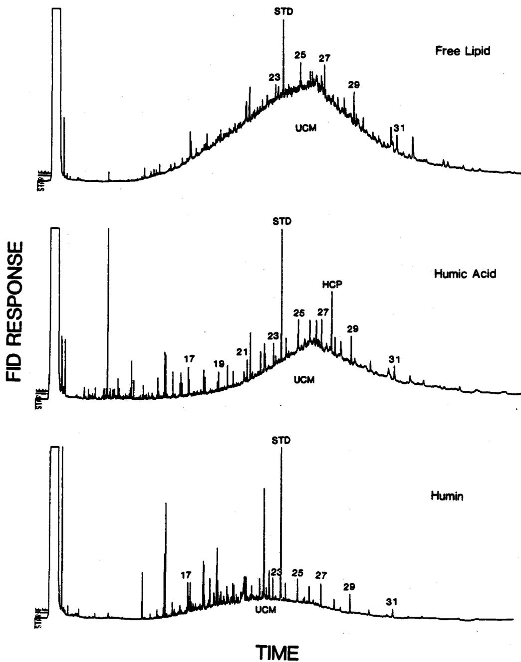
Figure 13. Capillary GC-FID chromatograms of FL, HA, and HU fractions of sample NB(0-3). STD - co-injection standard, perdeuterated tetracosane; UCM - unresolved complex mixture.
