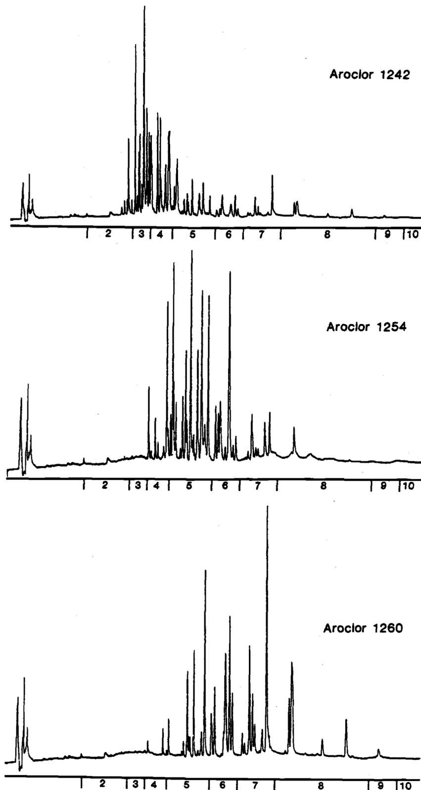
Figure 7. Capillary GC-ECD chromatograms of Aroclors 1242, 1254, and 1260
