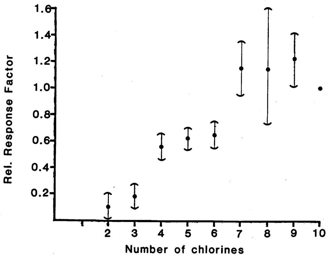
Figure 4. Response factors of PCB homologs (relative to decachlorobiphenyl) vs. chlorine content
