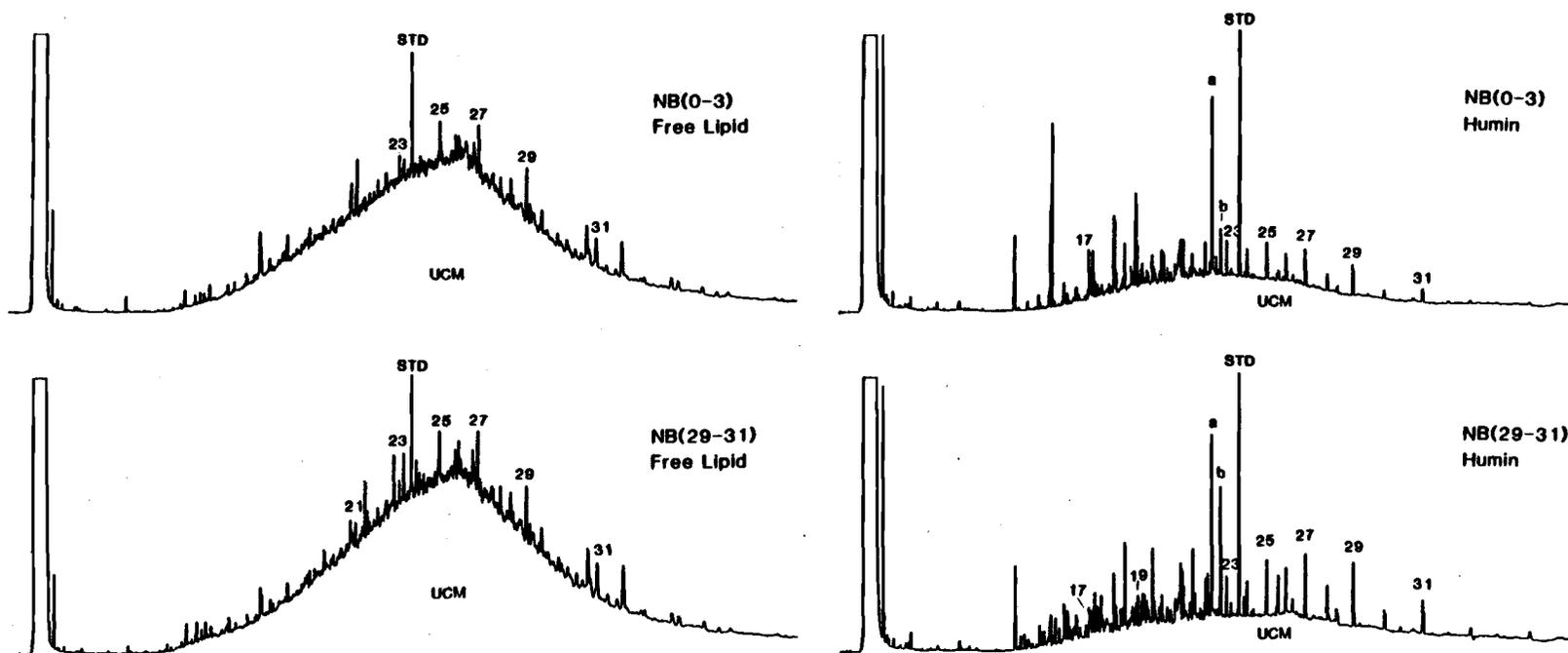
Figure 18. Capillary GC-FID chromatograms of saturated hydrocarbons in FL and HU fractions of samples NB(0-3) and NB(29-31). Peaks a and b discussed in text. See legend in Figure 13.
