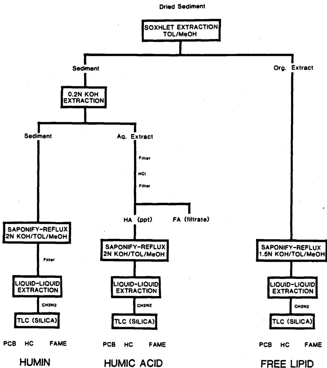
Figure 2. Schematic diagram of selective extraction procedure
