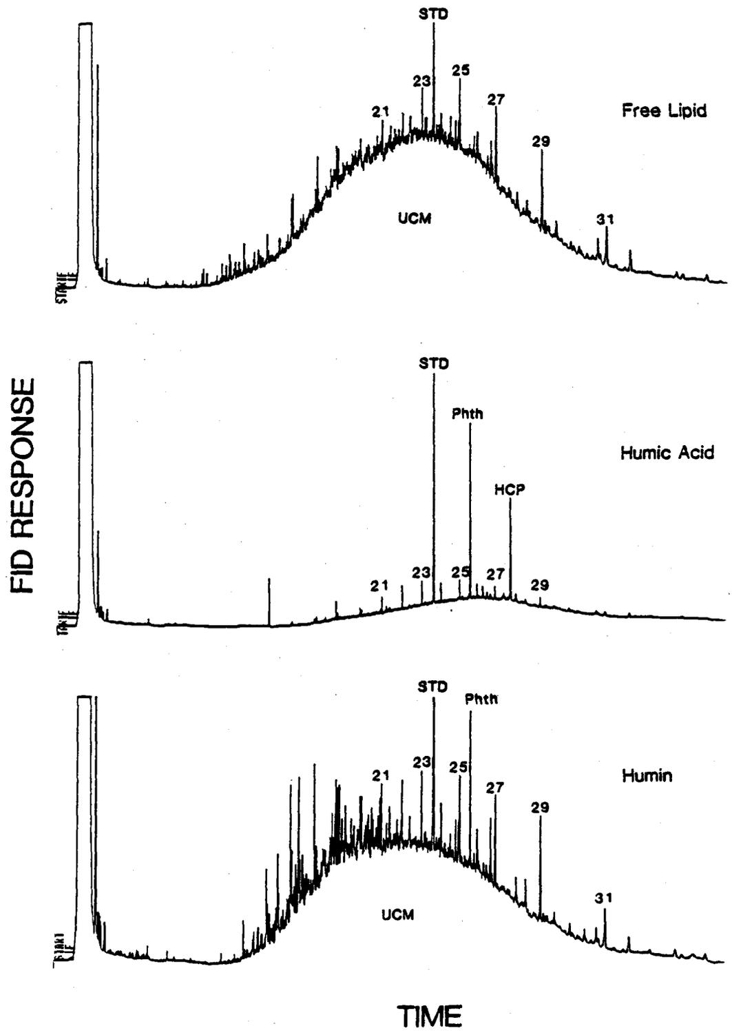
Figure 15. Capillary GC-FID chromatograms of FL, HA, and HU fractions of sample HR. See legend of Figure 13. Phth - C<sub>8</sub>-phthalate. Aromatic peaks are prevalent before C<sub>21</sub> in FL and HU fractions.
