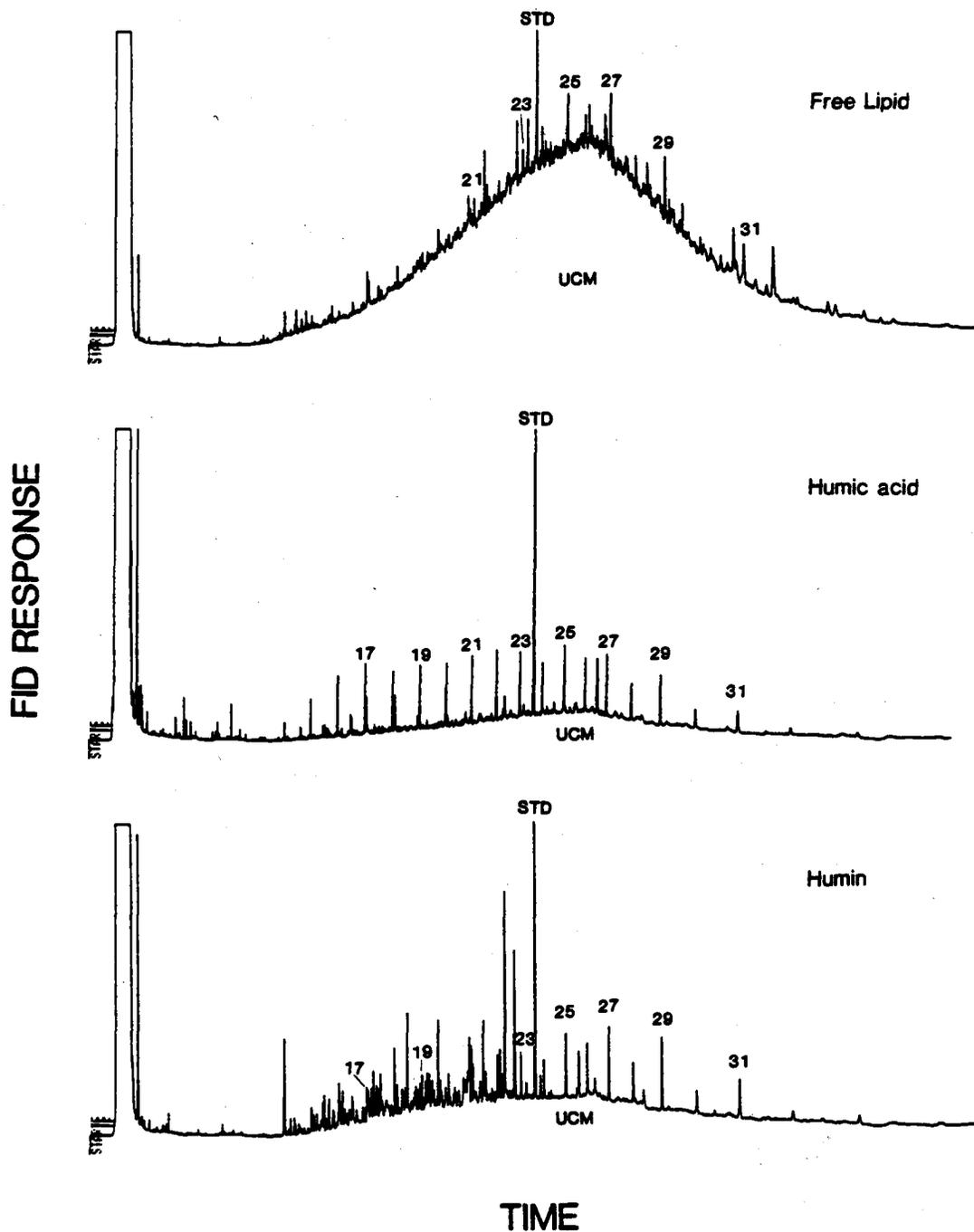
Figure 14. Capillary GC-FID chromatograms of FL, HA, and HU fractions of sample NB(29-31). See legend of Figure 13.
