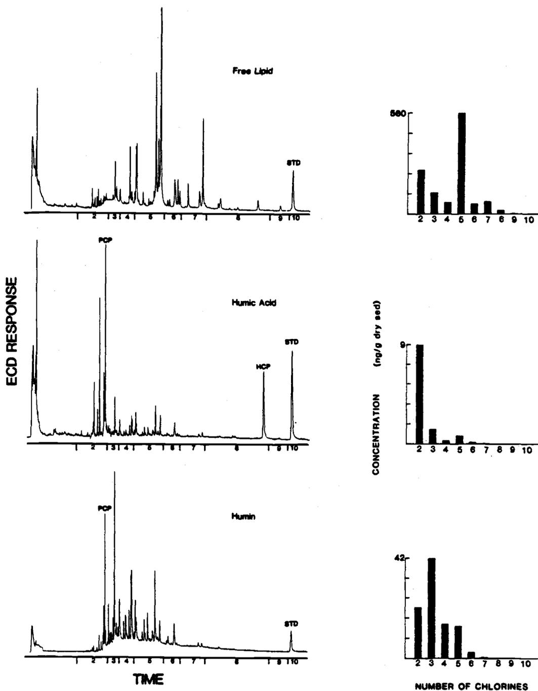
Figure 8. Capillary GC-ECD chromatograms of FL, HA, and HU fractions of sample NB(0-3). STD - co-injection standard, decachlorobiphenyl; PCP - pentachlorophenol (as methyl ether derivative); HCP - hexachlorophene (as dimethyl ether derivative). Homolog group concentrations, corrected with response factors, are presented in histograms.
