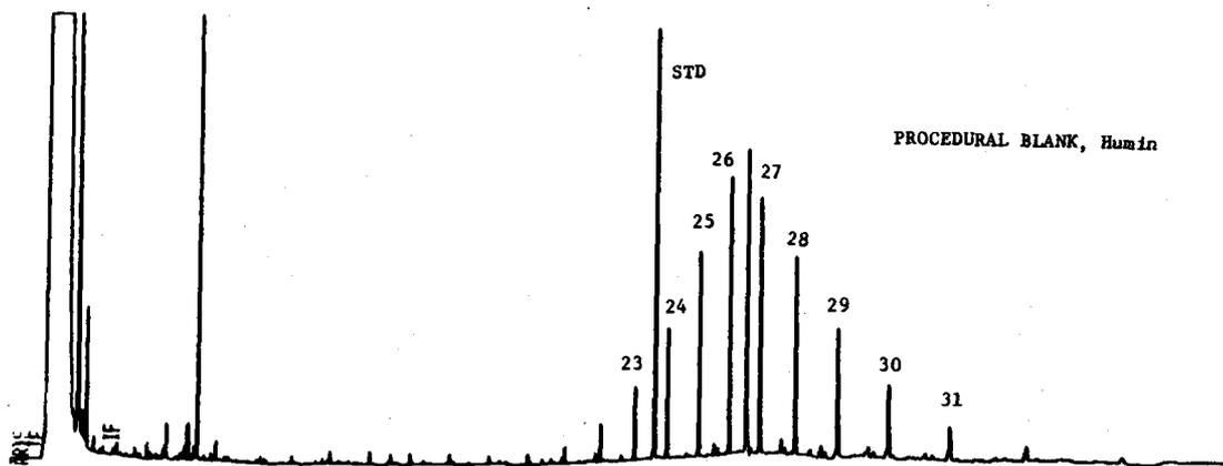
Figure 2A. GC-FID chromatograms of procedural blanks, Humic Acid and Humic Acid (hydrocarbon fractions)
