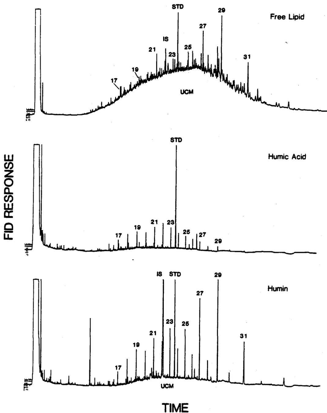
Figure 16. Capillary GC-FID chromatograms of FL, HA, and HU fractions of sample LA. STD - co-injection standard, per-deuterated tetracosane; IS - internal standard, *p*-terphenyl; UCM - unresolved complex mixture.
