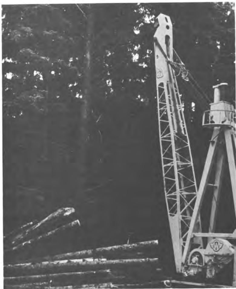
Figure 7. The Washington 98 thinning yarder bringing in a turn of logs from a steep hillside.
