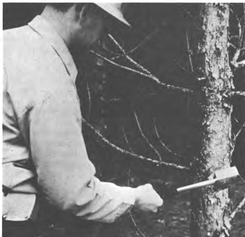
Figure 1. The Hypo-hatchet in operation, thinning lodgepole pine.
