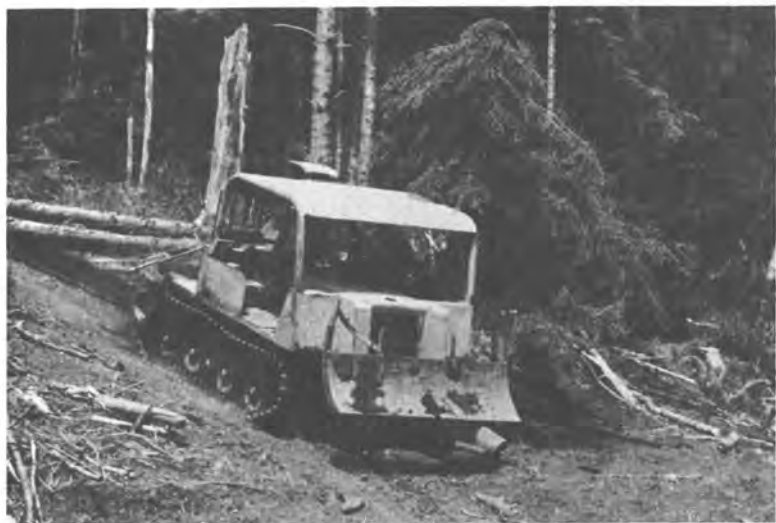
Figure 3. The Skagit Hustler with a turn of logs in a pretrailed thinning operation.
