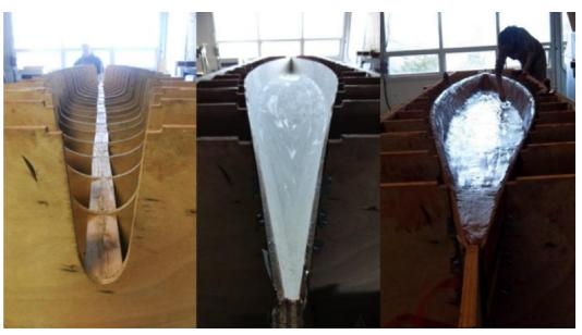
**FIGURE 1: Hull Construction Stages**
