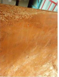
Figure 5: Inside view of crack This crack opens up and leaks severely when put in tension or in the water. The top of the canoe is in compression in this photo, which makes it appear minor.
