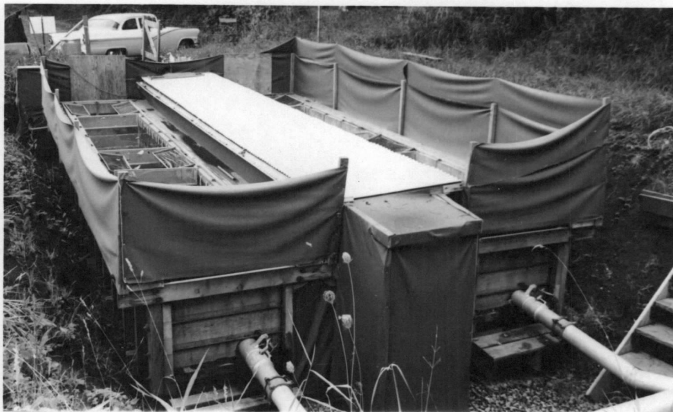
Figure 1. Paired stream aquaria. Walls facing the central observation chamber are glass.
