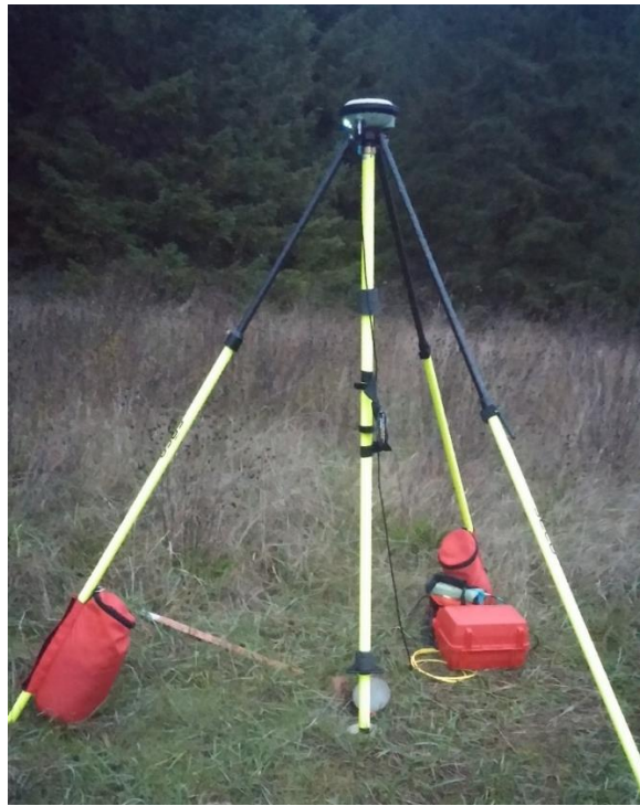
Figure 8. Example photograph of a static GNSS setup with the equipment used in this study (Note this photograph was acquired at different field site)
