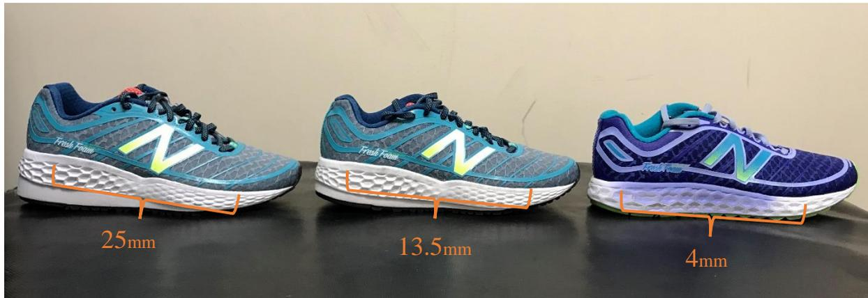
An image with each shoe condition used in the study. Starting on the left: the large drop cushioned shoe, the traditional cushioned shoe, and the low drop cushioned shoe. Brackets designate the heel to toe drop in millimeters. A heel to toe drop is the difference between the forefoot cushion height and the rearfoot cushion height.
