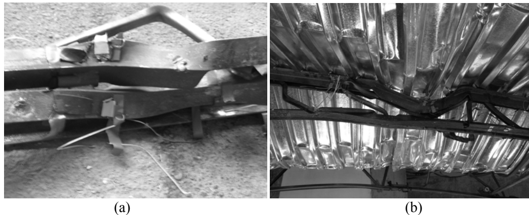
Figure 83: Failed Members, (a) Pitched Test Center Joist (b) Flat Test Center Joist
