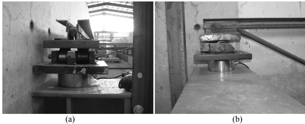
Figure 41: Load Cell Installation, (a) End View (b) Side View
