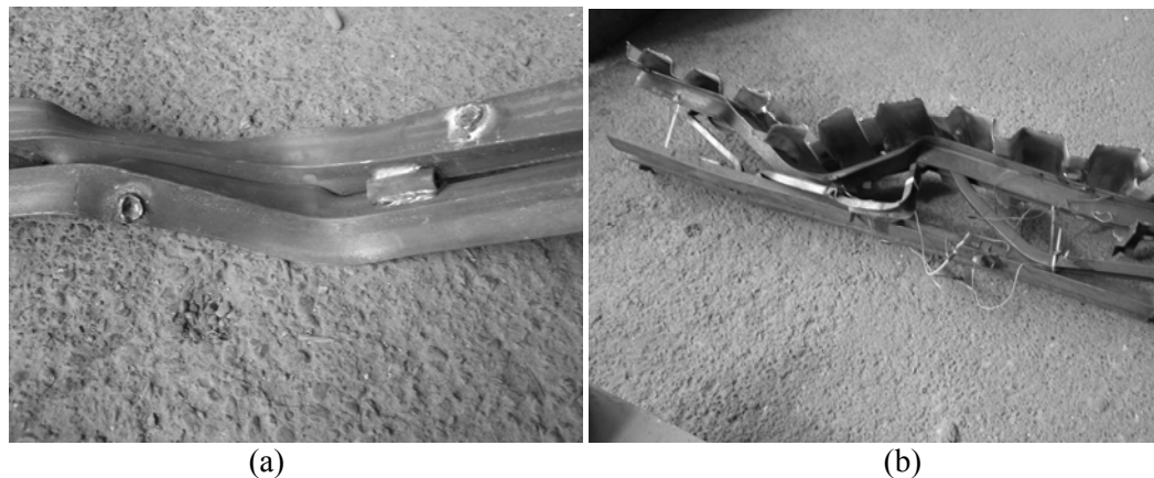
Figure 82: Failed Members, (a) Flat Test Side Joist (b) Flat Test Center Joist
