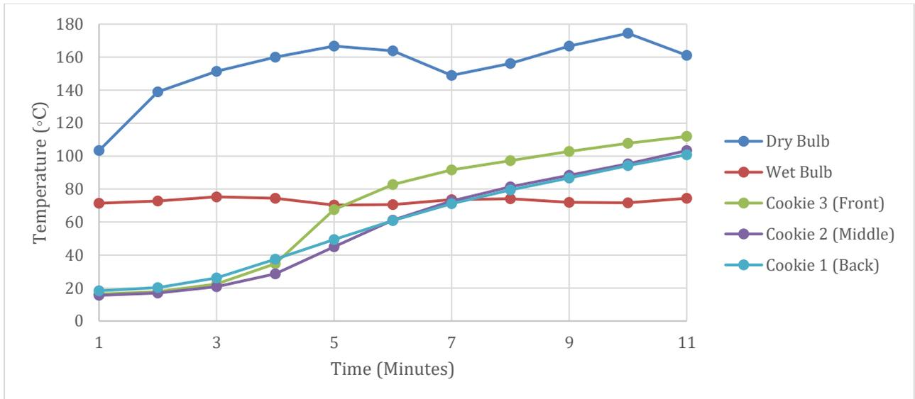
Figure 2.1. Temperature profiles of oven (dry and wet bulb) and internal cookies during baking process (325F, 11 min).
