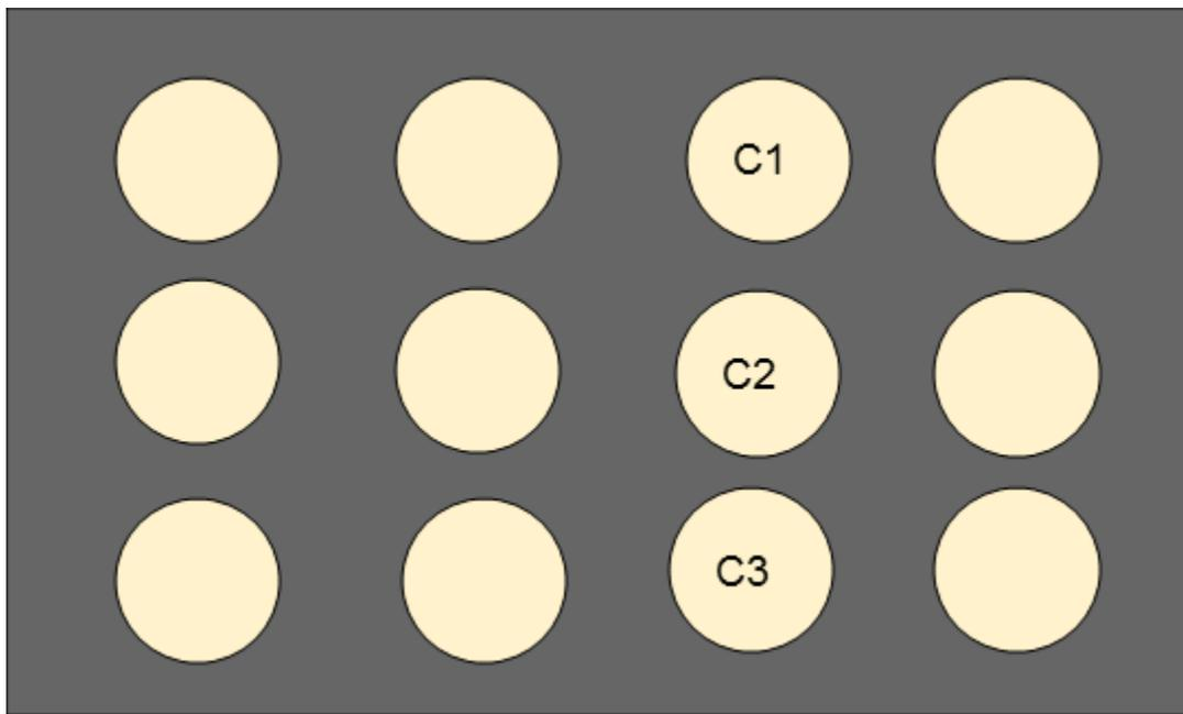
Figure 3.1: Cookie placement and thermocouple positions from back of oven (C1) to front of oven (C3).
