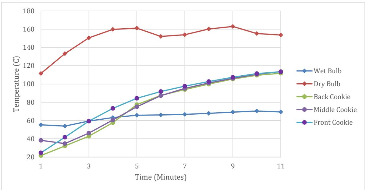
Figure 3.2: Mean baking temperature profiles for the oven chamber (dry bulb and wet bulb) and internal cookie temperature at the back, middle, and front of the oven baked at 163°C for 11 min.
