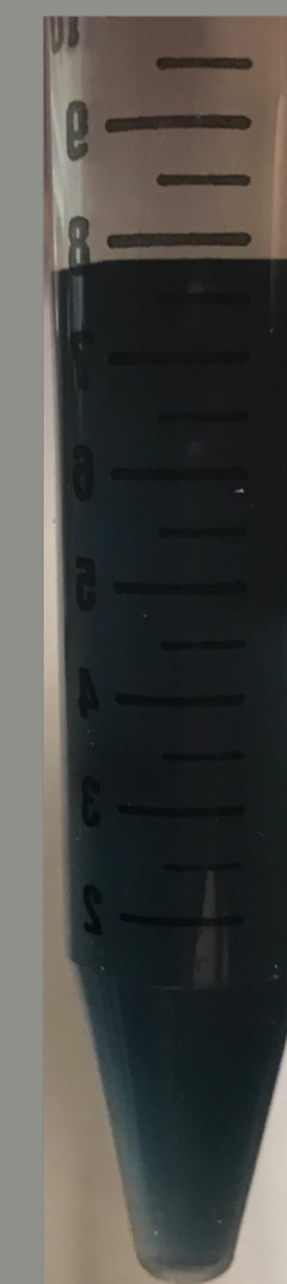
Figure 5. A nanostar suspension after synthesis at 5°C. This suspension is analyzed with a UV/Vis spectrophotometer. Magnifying this by several thousands of times is how you would see the structure and geometry of the nanostars.
