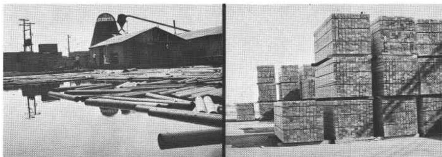
Figure 11. Peeler cores (left) are sawed at White City into 8-foot studs (right), a popular item for residential construction.
