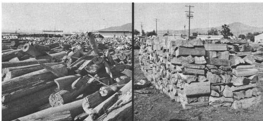
Figure 12. Split peeler cores (left) become fuel (right).
