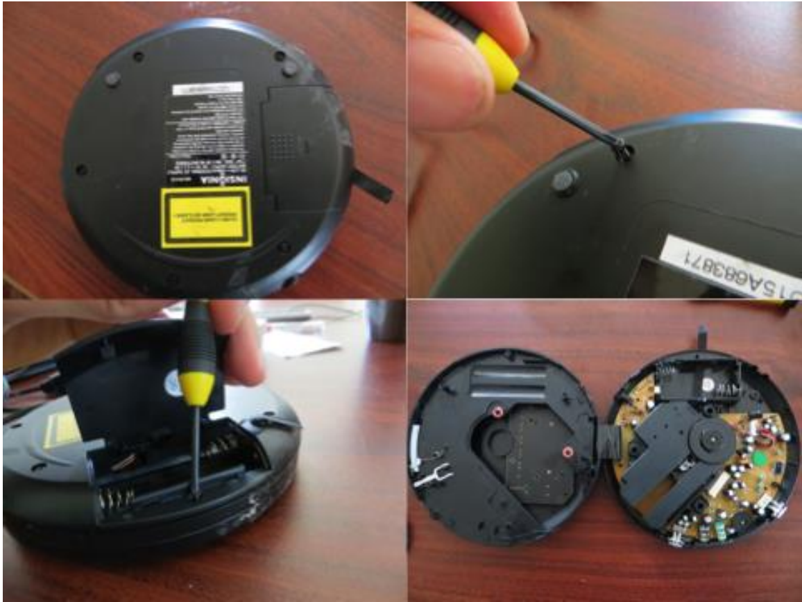
Figure 1. Each screw is removed from the CD player to gain access to the electrical components of the unit. Most CD players have the screws located on the back of the unit, yet some also have them on the CD deck. Make sure all screws are removed before taking off the shell. Carefully pull apart the unit and note that the data ribbon between the integrated circuit board and the main circuit board will still be connected.
