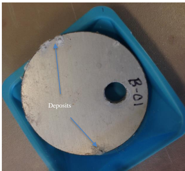
Figure 4.3. Deposit spots distribution on pre-filmed coupon from first month
