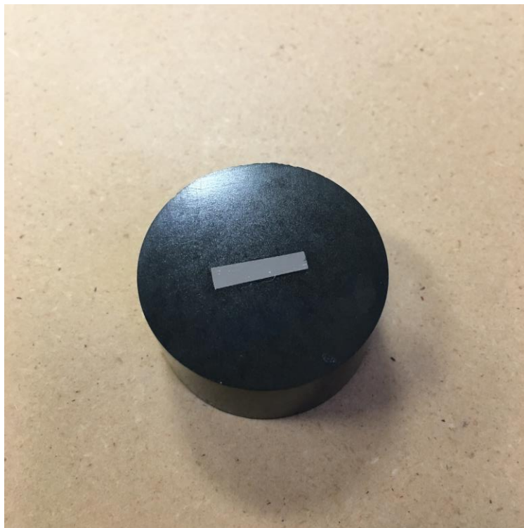
Figure 3.4. Prepared cross-section sample from a pre-filmed coupon
