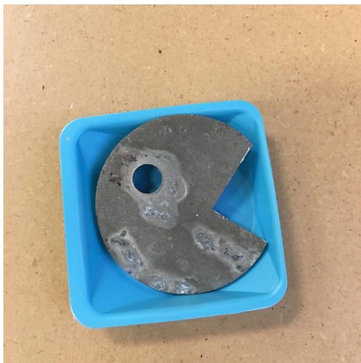
Figure 3.5. A non-pre-filmed coupon after a sectioning
