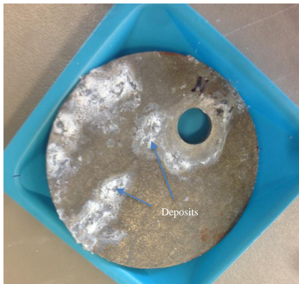
Figure 4.4. Deposit spots distribution on non-pre-filmed coupon from first month
