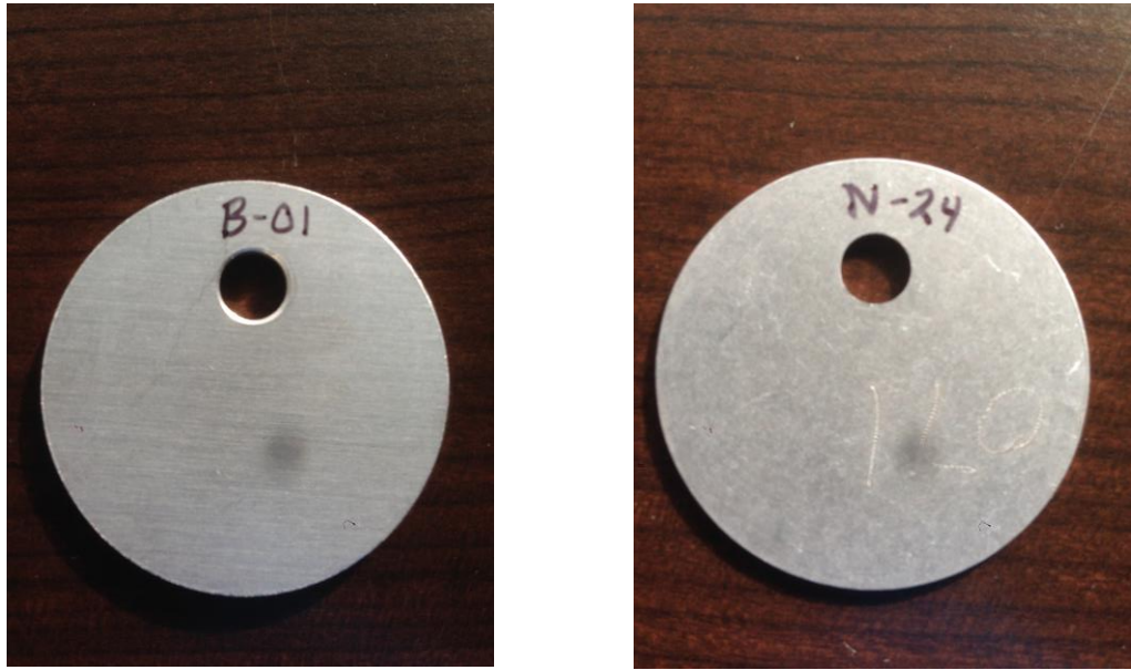
Figure 3.2. Boehmite pre-filmed coupon (left) and non-pre-filmed coupon (right)
