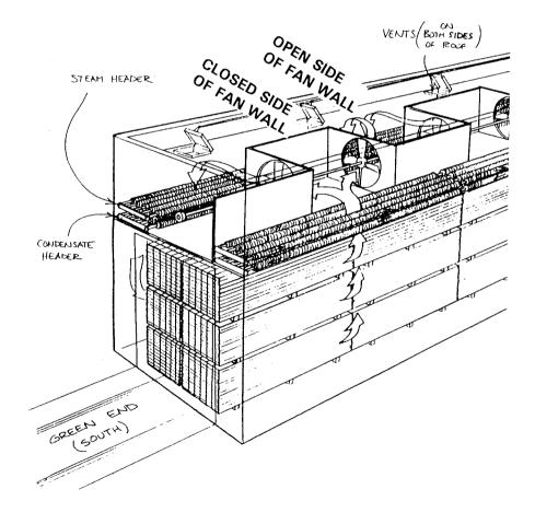
FIGURE 1. Open and closed sides of fan wall.
