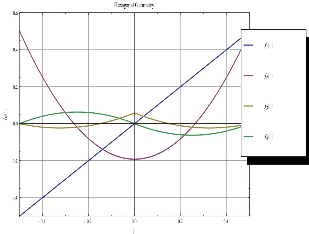
**Figure 3.7 Polynomial expansion functions in hexagonal geometry**
