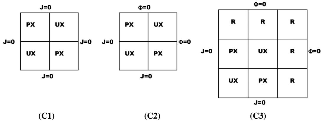
**Figure 3.8 UO<sub>2</sub>-MOX (C1, C2) and UO<sub>2</sub>-MOX-water (C3) configurations**
