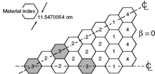
**Figure 3.9 The hexagonal IAEA 2-D reactor.**
