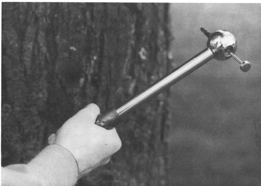
Figure 12.—An increment hammer is used to obtain a sample of a tree's outer inch.
