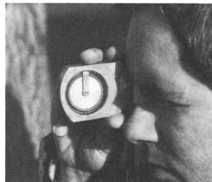
Figure 6.—(right) The clinometer has a sighting hole and a suspended circular scale.
