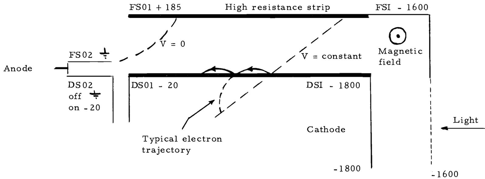
Figure 7. Schematic diagram of the modified magnetic electron multiplier.
