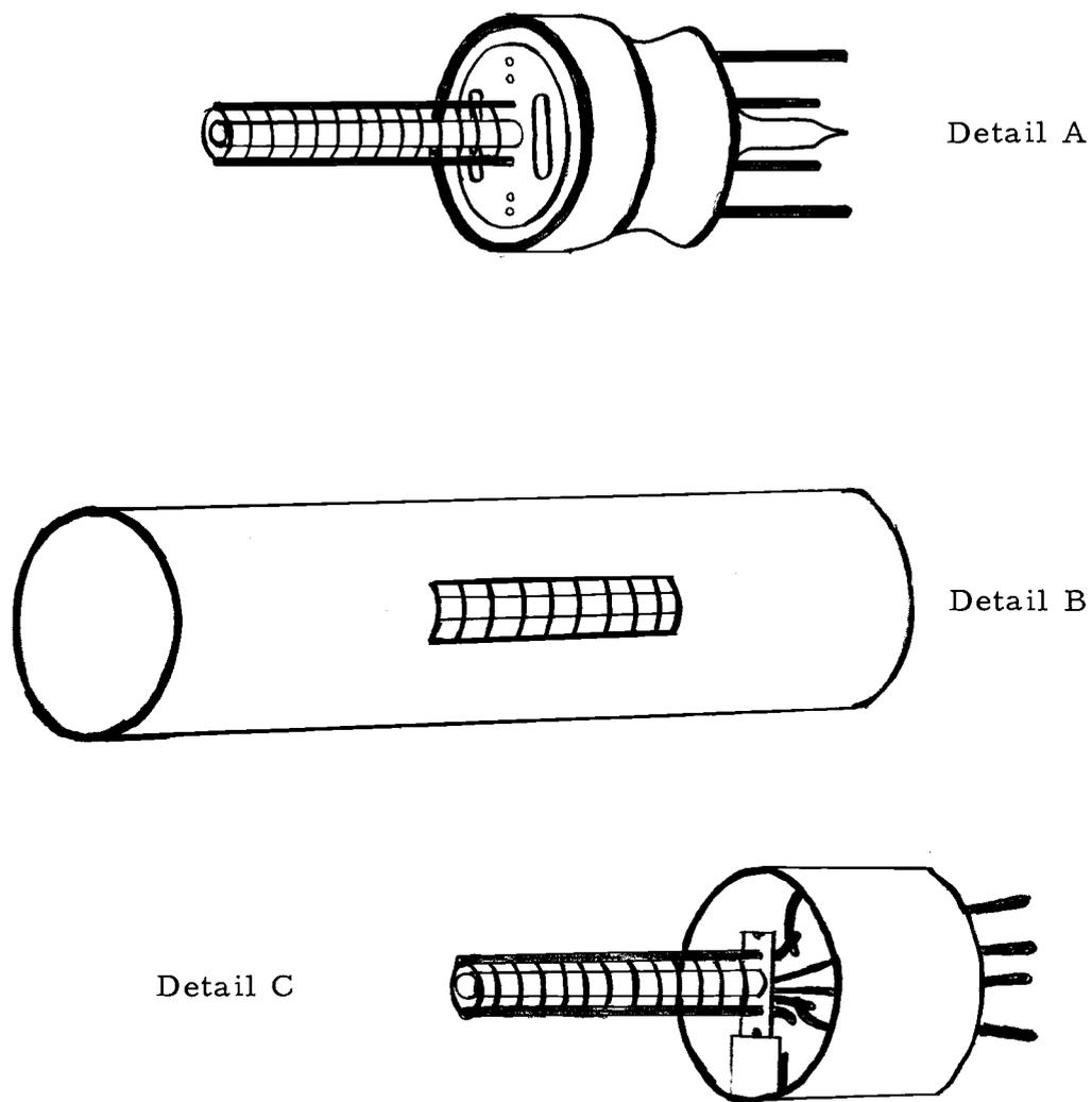
Figure 5. Electron gun used in argon experiment (Detail A). Excitation enclosure (Detail B) and electron gun (Detail C) used in the krypton experiment.
