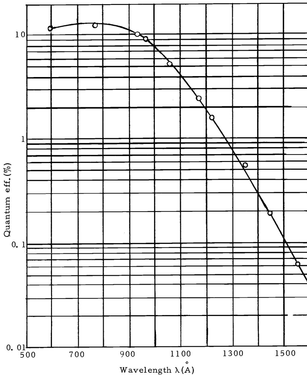
Figure 6. Quantum efficiency of the Bendix Model M308 magnetic electron multiplier. (Reprinted from the M308 Instruction Manual.)
