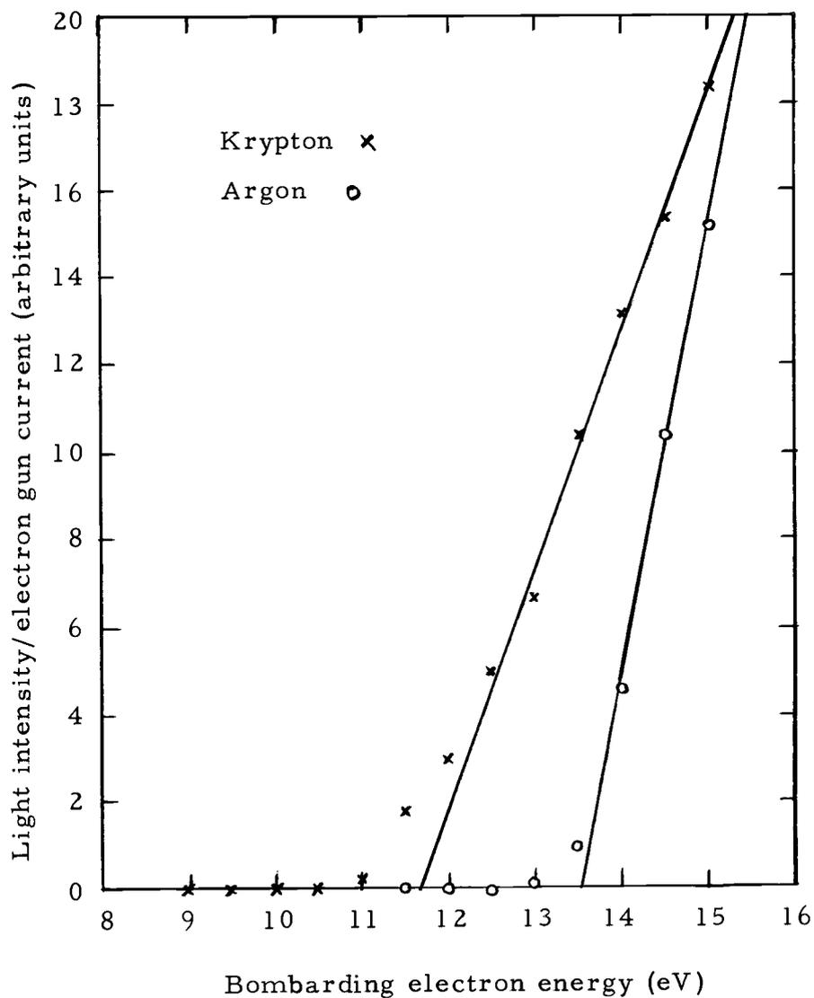
Figure 13. Threshold curves for excitation of the first excited  $J = 1$  ( $^3P_1$ ) levels in argon and krypton by electron bombardment.
