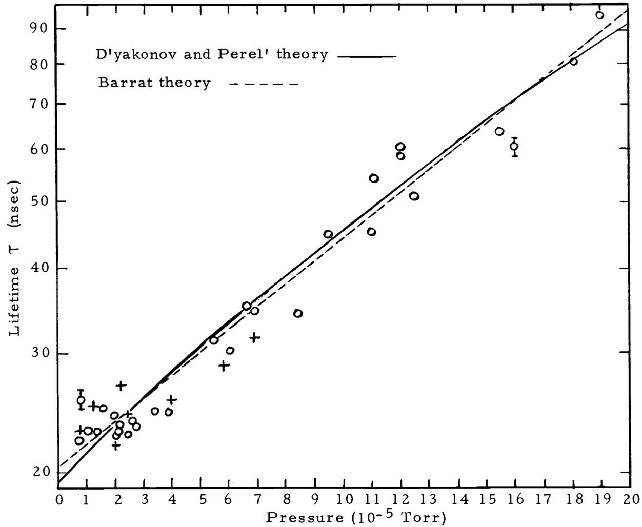
Figure 16. Imprisoned lifetime  $\tau$  for the argon decay as a function of pressure. The open circles and crosses indicate data points taken with the center of the electron gun 3.5 and 2.0 cm, respectively, from the lithium fluoride window. Fits to the data taken at 3.5 cm are shown for the theories by Barrat, and D'yakonov and Perel'.
