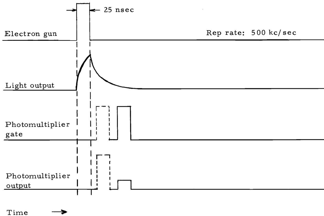
Figure 1. Sequence of events in modified delayed-coincidence method. The numbers shown are typical values used in the argon experiment.
