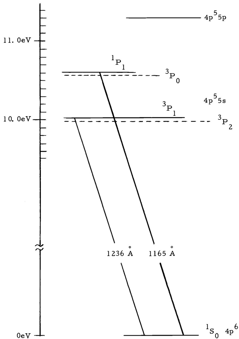
Figure 17. Partial energy-level diagram for krypton.
