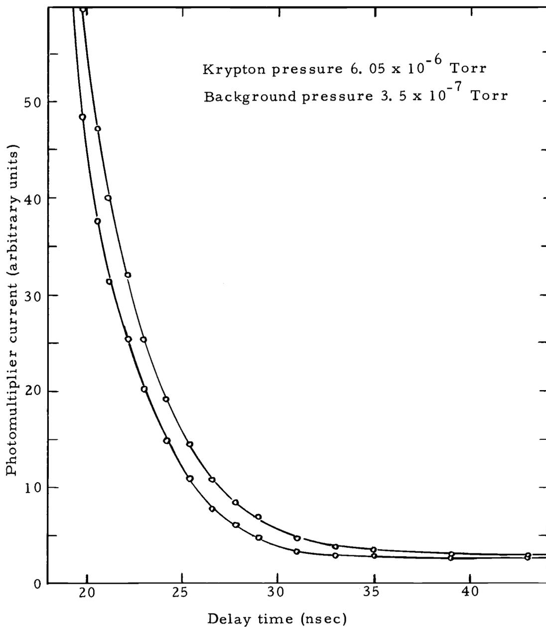
Figure 18. Typical plots of photomultiplier current as a function of delay time. The lower curve represents the decaying light signal from the system at background pressures and the upper curve represents the sum of the lower curve and the signal due to krypton.
