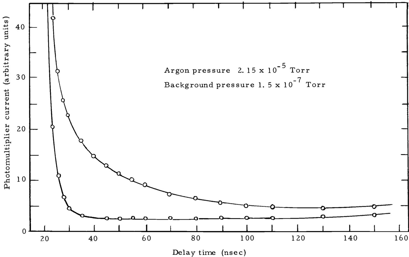
Figure 14. Typical plots of photomultiplier current as a function of delay time. The lower curve represents the decaying light signal from the system at background pressures and the upper curve represents the sum of the lower curve and the signal due to argon.
