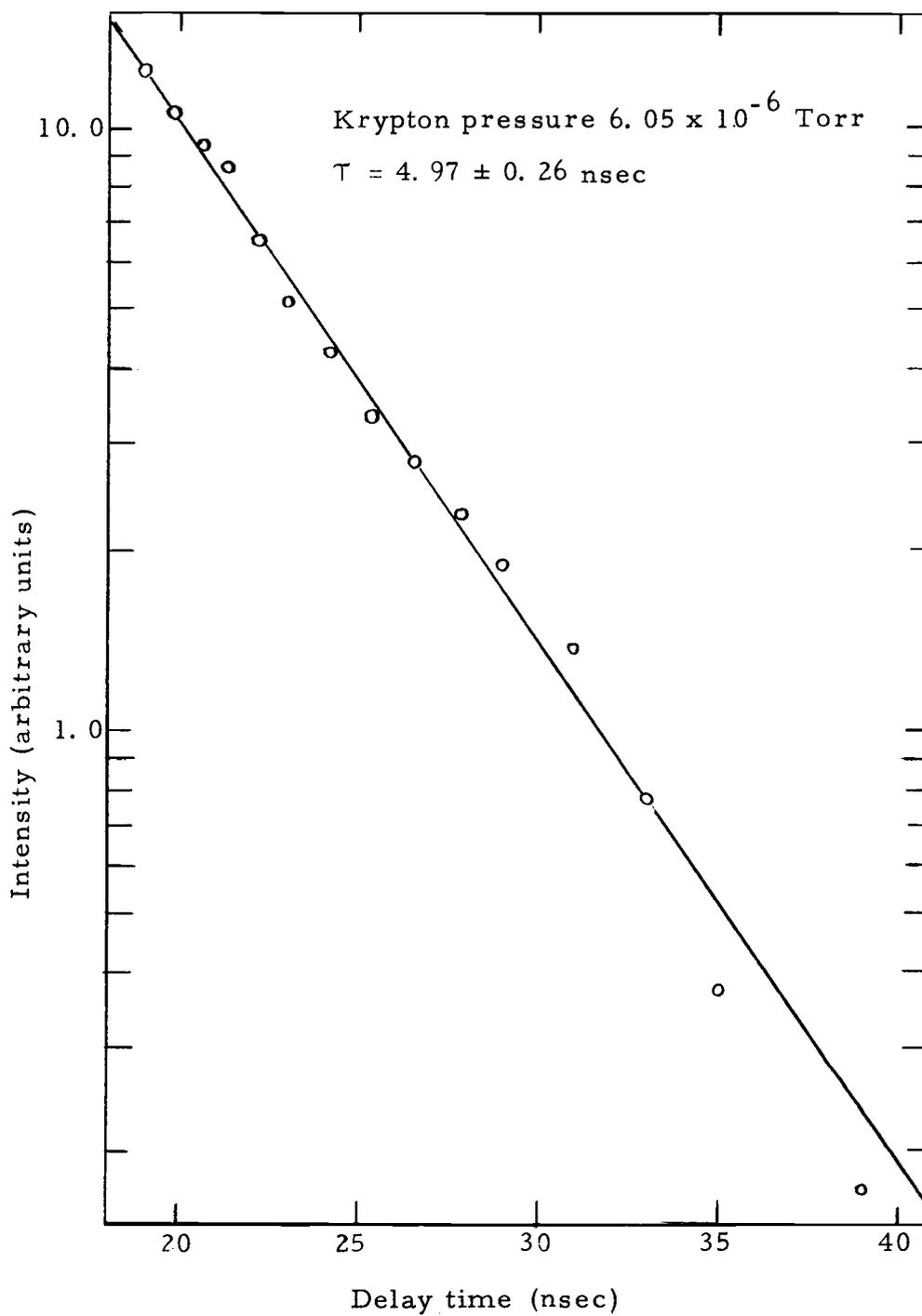
Figure 19. Typical krypton-decay curve.
