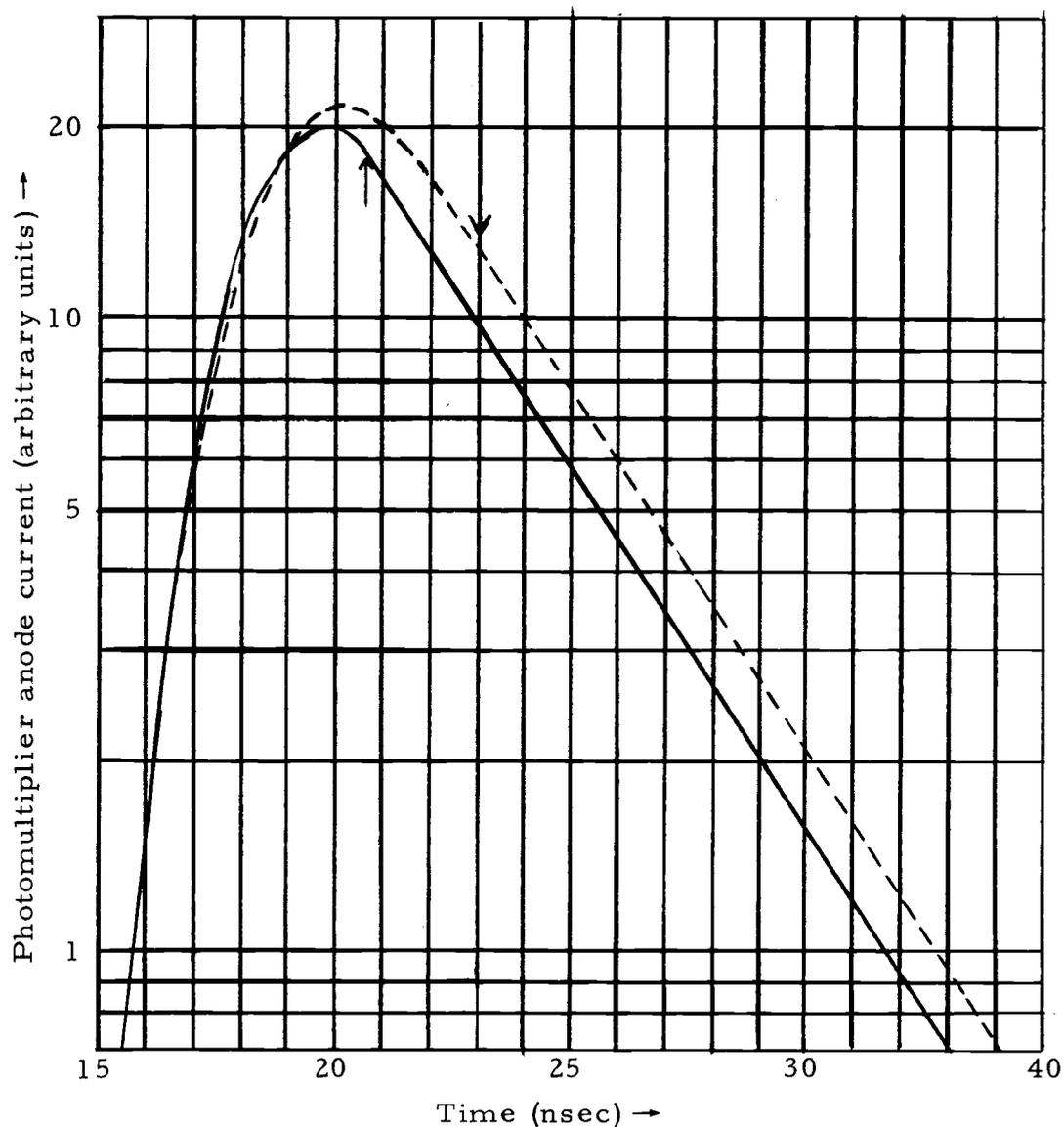
Figure 9. Time dependence of the photomultiplier anode current for an exponentially decaying light signal incident at  $t = 0$ . For the solid curve, a rectangular-shaped secondary electron pulse is assumed; the arrow in the figure depicts the time after which the anode current decays exponentially. For the dotted curve, a gaussian shaped pulse is assumed; the arrow depicts the time after which the anode current differs by less than 1% from an exponential decay.
