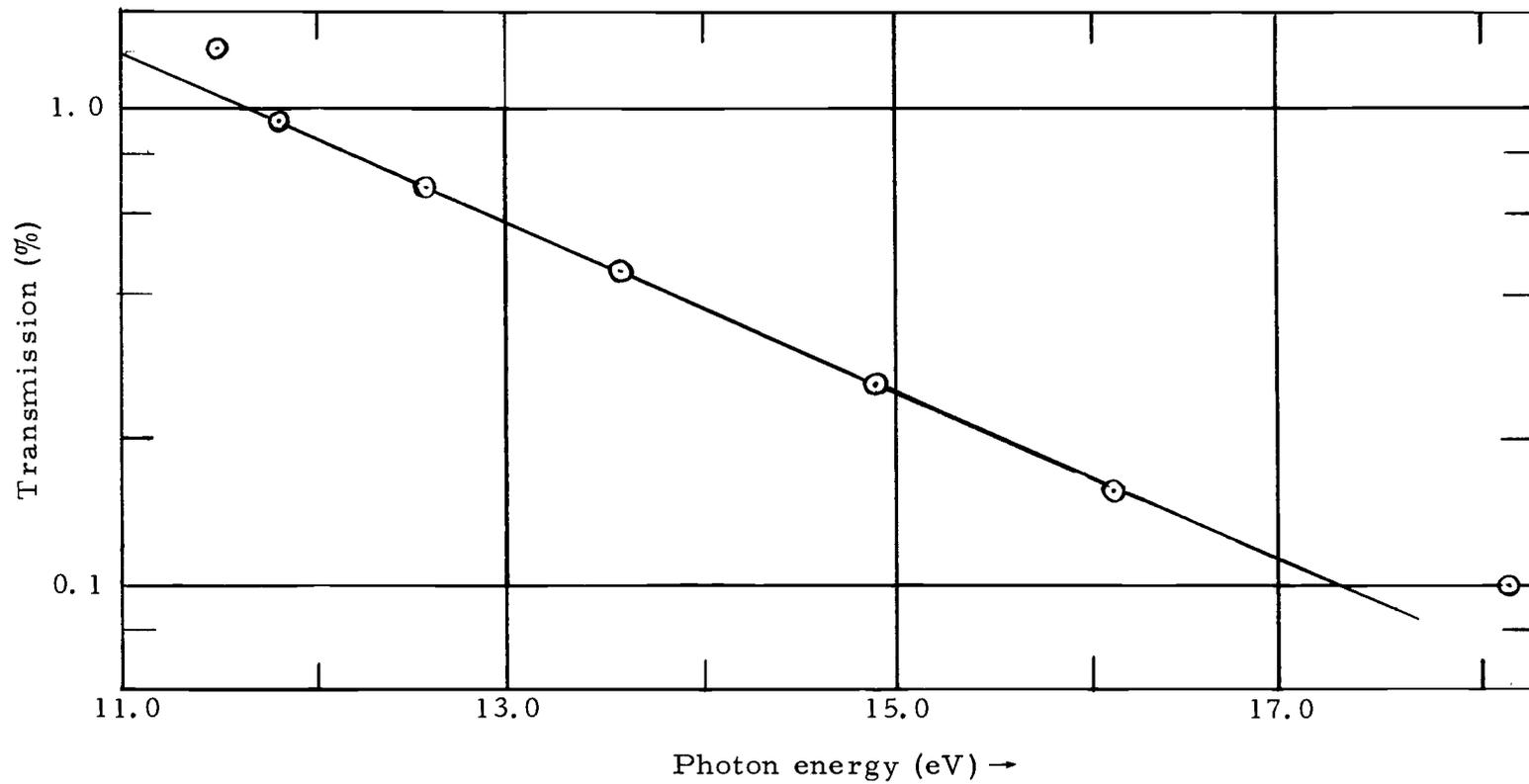
Figure 12. Transmission of a 420 Å thick aluminum oxide film as a function of photon energy.
