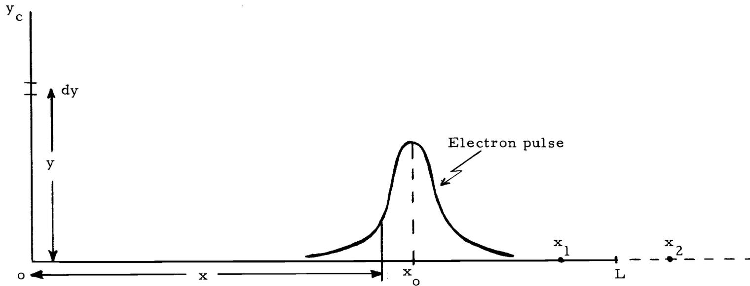
Figure 8. Coordinates used in the discussion of electron multiplication in the magnetic electron multiplier.
