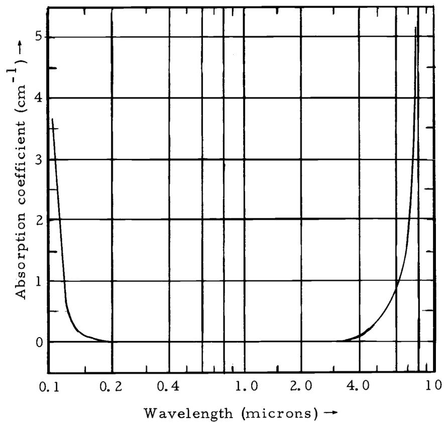
Figure 11. Wavelength dependence of the absorption coefficient of lithium fluoride.
