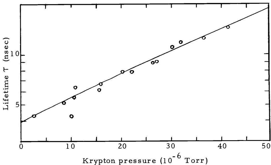
Figure 21. Imprisoned lifetime  $\tau$ , for the krypton decay, as a function of pressure. The solid curve represents a fit of the data to the theory of D'yakonov and Perel'.
