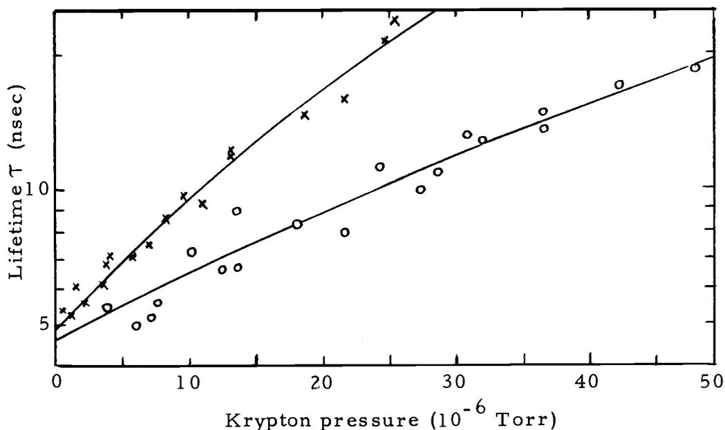
Figure 20. Imprisoned lifetime  $\tau$ , for the krypton decay, as a function of pressure. The solid curve represents fit of the data to the theory of D'yakonov and Perel'. The excitation enclosure used for the lower set of data was considerably smaller than that used for the upper set of data.
