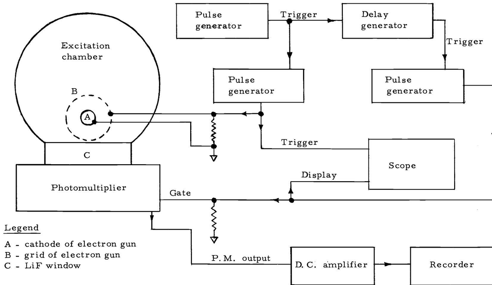
Figure 2. Schematic diagram of the apparatus.
