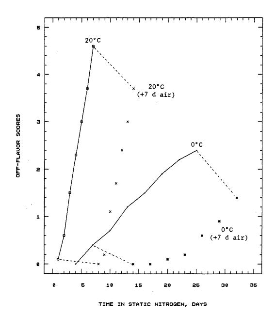
Fig. III.28. Off-flavor (scale 0 to 8, 0 = no off-flavor) development and partial reversal in 'Bartlett' pears under static  $N_2$  at 0° and 20°C, followed by 7 days in air. Each point represents the mean of 10 observations.
