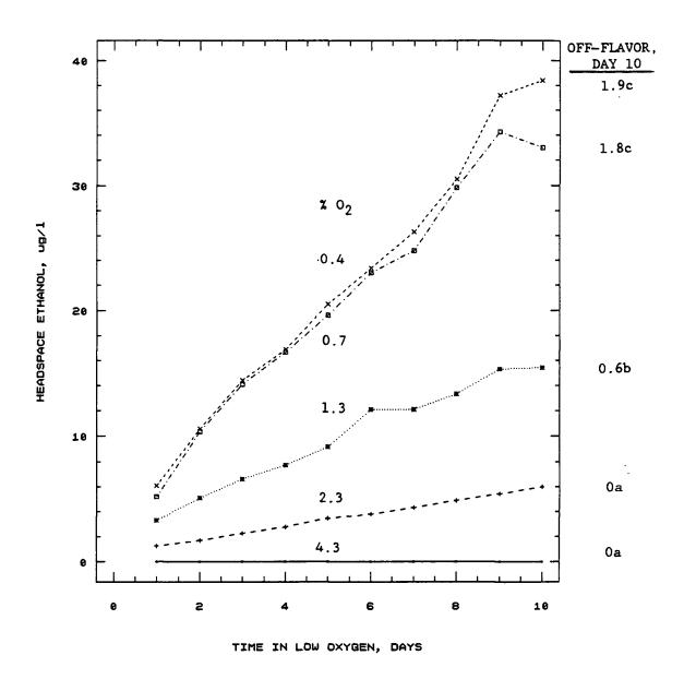
Fig. VI.9. Headspace ethanol of 'Marion' blackberries in  $0^{\circ}\text{C}$  storage with continuous flow (10 ml/min) low- $0_2$  atmospheres; and off-flavor scores (0 to 8, 0 = no off flavor) after 10 days. Each point represents the mean of 2 observations for ethanol and 10 observations for off-flavor scores by the sensory panel. Mean separation by Duncan's multiple range test, 5% level.
