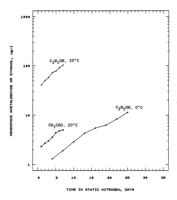
Fig. III.10. Headspace acetaldehyde and ethanol of 'Granny Smith' apples under static N $_2$  at 0° and 20°C. Each point represents the mean of 3 observations. At 0°C, acetaldehyde was below detection limits (0.5 ug/l) at all sampling times.
