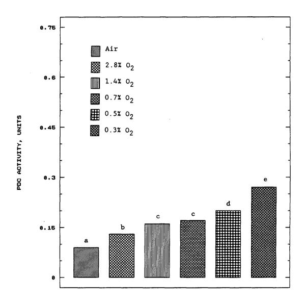
Fig. V.11. Pyruvate decarboxylase (PDC) activity of 'Anjou' pears after 24 days in air or controlled atmosphere storage at  $0^{\circ}C$ . Each bar represents the mean of 4 observations. Mean separation by Duncan's multiple range test, 5% level.
