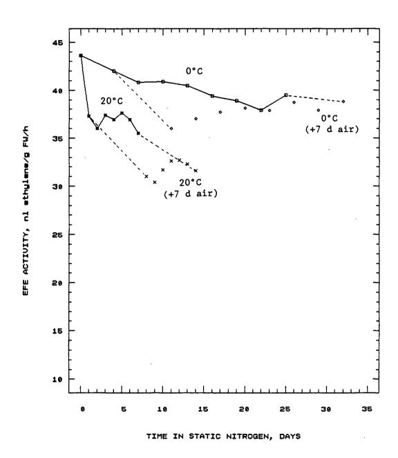
Fig. III.21. Ethylene forming enzyme (EFE) activity in 'Golden Delicious' apples under static  $\rm N_2$  at 0° and 20°C, followed by 7 days in air. Each point represents the mean of 3 observations.
