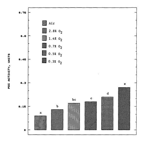
Fig. B.7. Pyruvate decarboxylase (PDC) activity of 'Anjou' pears after 24 days in air or controlled atmosphere storage at  $0^{\circ}$ C, followed by 7 days in air. Each bar represents the mean of 4 observations. Mean separation by Duncan's multiple range test, 5% level.
