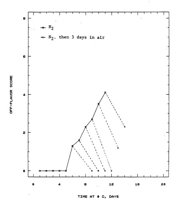
Fig. VI.11. Off-flavor (scale 0 to 8, 0 = no off flavor) development of 'Italian' plums in static  $N_2$  at 0°C, and partial reversal by transfer to air storage for 3 days. Each point represents the mean of 10 observations.
