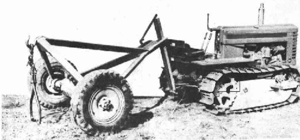
Figure 1.--Jack-knife sulky ready for hooking on to a load.
