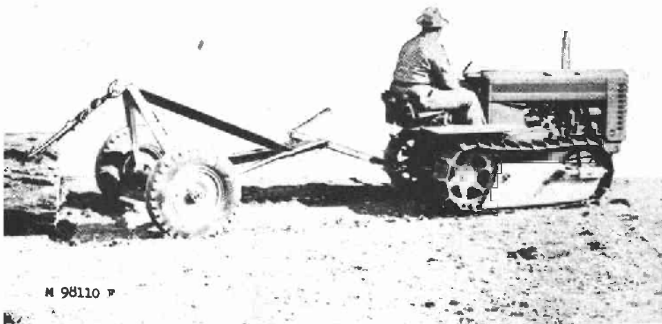
Figure 2.--Sulky tongue being pulled straight to raise the load.
