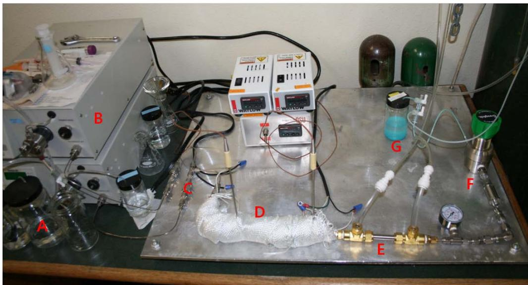
**Fig. S1.** Photograph of the CFMA system used for the high-rate synthesis of Cu-BTC. (A) Precursors in solutions, (B) HPLC pumps, (C) Mixing zone, (D) Reaction zone, (E) Cooling zone, (F) Back-pressure regulator, and (G) Collecting zone.
