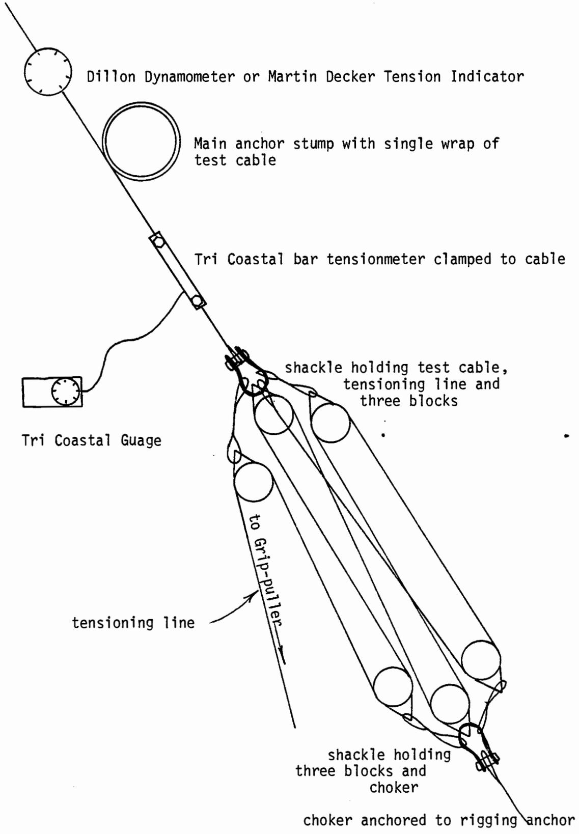
Figure 6. Block rigging configuration
