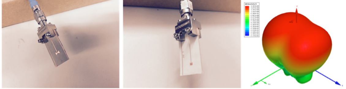
Figure 2.2: Broadband 56-62GHz bowtie and 55-57GHz patch antennas fabricated on Rogers substrate and connectorized with V-band end launches; Simulated radiation pattern of the bowtie antenna.
