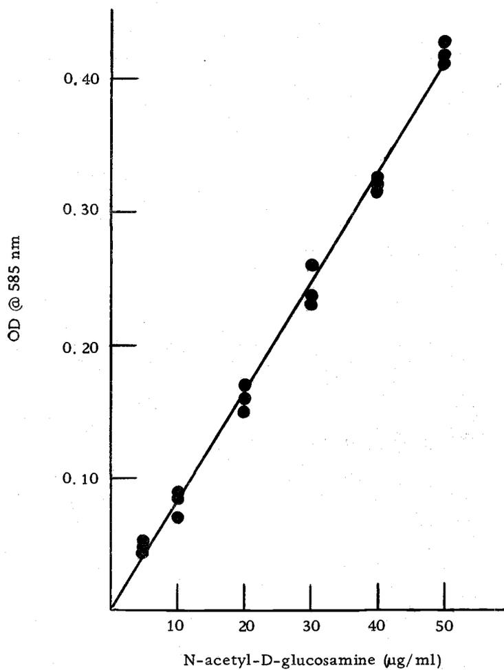
Figure 1. Standard curve of N-acetyl-D-glucosamine. Six concentrations of NAG were utilized to yield a standard curve for the conversion of OD readings at 585 nm to µg NAG produced. The assay was the Reissig et al. Modification of the Morgan-Elson colorimetric assay for N-acetyl-D-hexosamine. Correlation coefficient is 0.9974;  $m = 0.00815$ ;  $b = 0.00061$ .
