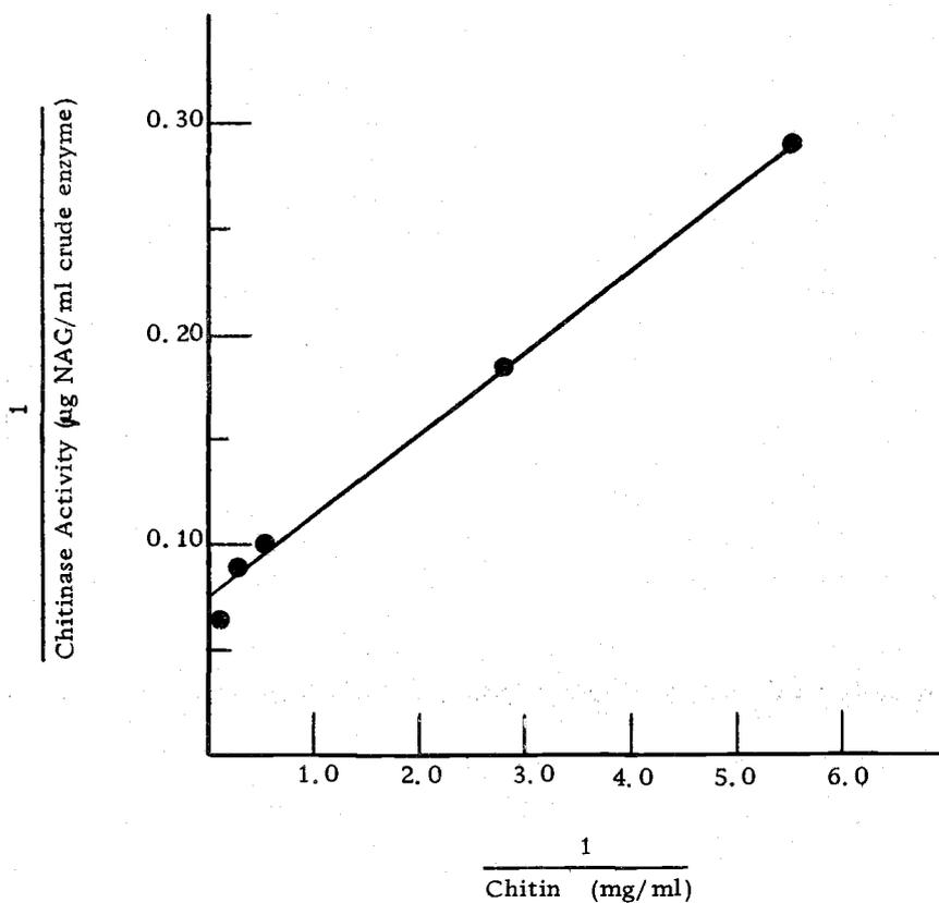
Figure 6. Effect of chitin concentration on enzyme activity. Reciprocal of  $\mu\text{g}$  N-acetyl-D-glucosamine produced per ml crude enzyme per unit time v. the reciprocal of chitin concentration (mg/ml). Correlation coefficient is 0.9964;  $m = 0.367$ ;  $b = 0.0732$ ;  $V_{\max} = 13.65 \mu\text{g NAC/ml enzyme} \cdot t$ ;  $K_m = 0.50 \text{ mg/ml chitin}$ . Incubation time was 24 h.
