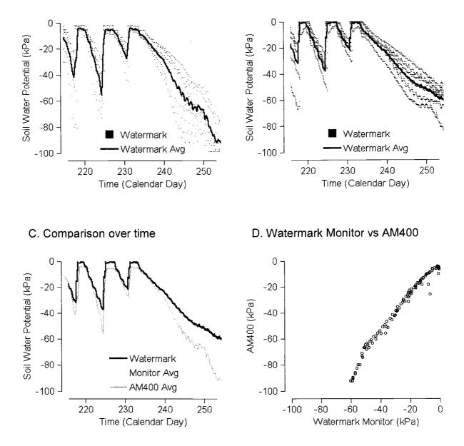
Figure 1. Response of Watermark soil moisture sensors to irrigation events and the termination of irrigation as measured by an AM400 Hansen datalogger (A) and an Irrometer Watermark Monitor (B). The average readings of the an AM400 Hansen datalogger and an Irrometer Watermark Monitor are compared over time (C) and over the measured range of soil water potential (D), Malheur Experiment Station, Oregon State University, Ontario, OR, 2003.
