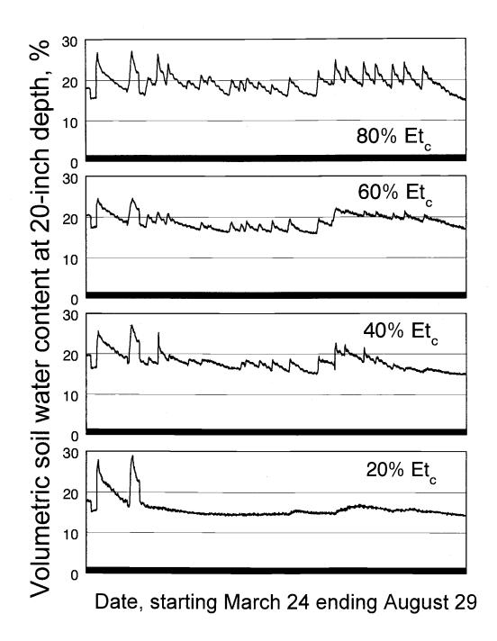
Figure 3. Soil moisture response to irrigation treatment in a drip-irrigated alfalfa seed field, Malheur Experiment Station, Oregon State University, Ontario, OR, 2003.
