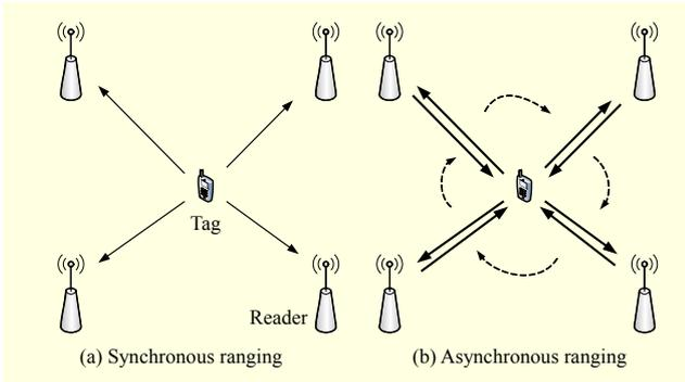
Fig. 1. Ranging architecture: (a) uses only one message for ranging but precise time synchronization is needed, and (b) uses numerous messages for ranging.
