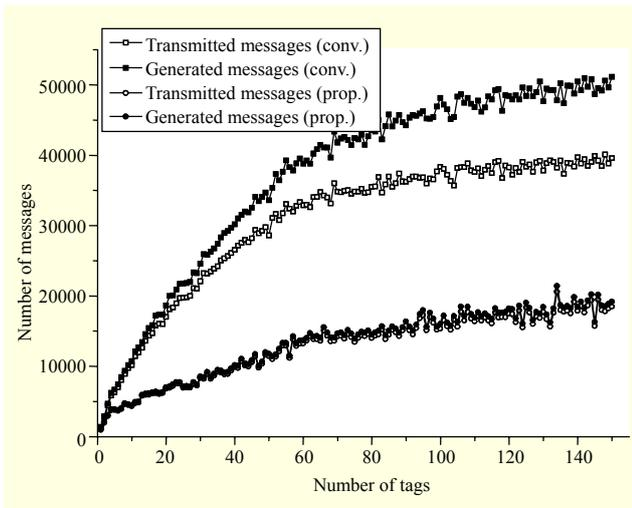
Fig. 2. Generated and transmitted messages in radio layer.
