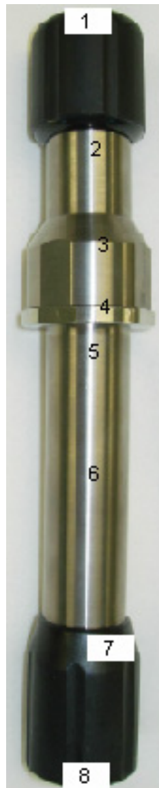
Figure 5: Exposure Points on 5mL Tungsten Pig, exposure points chosen on the 5mL Unit Dose Pig to find shielding effectiveness at thin points, seals and typical human contact points
