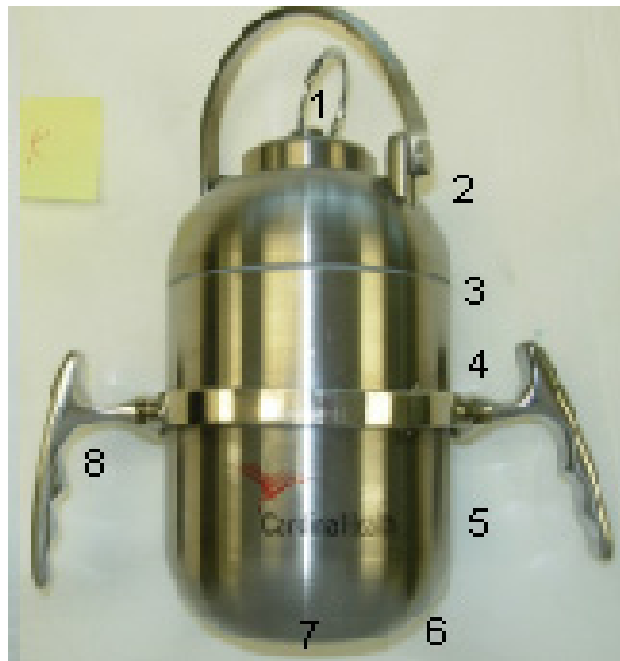
Figure 6: Exposure Points on 30mL PET Dispenser, exposure points chosen on the 30mL PET Dispenser to find shielding effectiveness at thin points, seals and typical human contact points.
