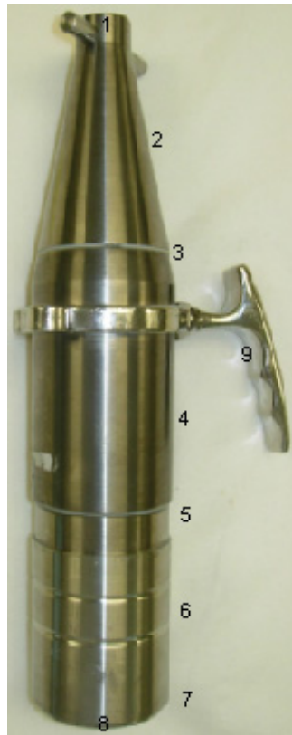
Figure 4: Exposure Points on 10mL PET Pig, exposure points chosen on the 10mL PET Pig to find shielding effectiveness at thin points, seals and typical human contact points.
