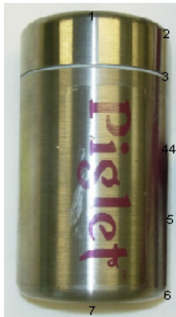
Figure 7: Exposure Points on Piglet, exposure points chosen on the Piglet to find shielding effectiveness at thin points, seals and typical human contact points.
