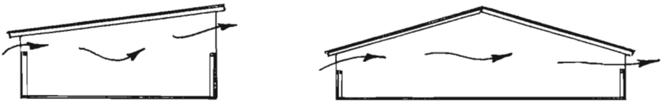
FIGURE 1. Make use of cross ventilation in summer.
